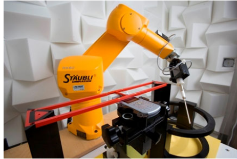
Figure 4-3 SPEAG Robotic System
