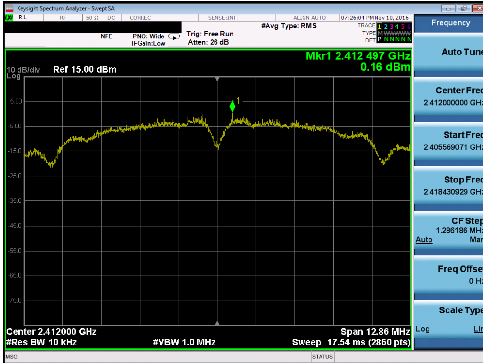
Plot 7-10. Power Spectral Density Plot (802.11b – Ch. 1)
