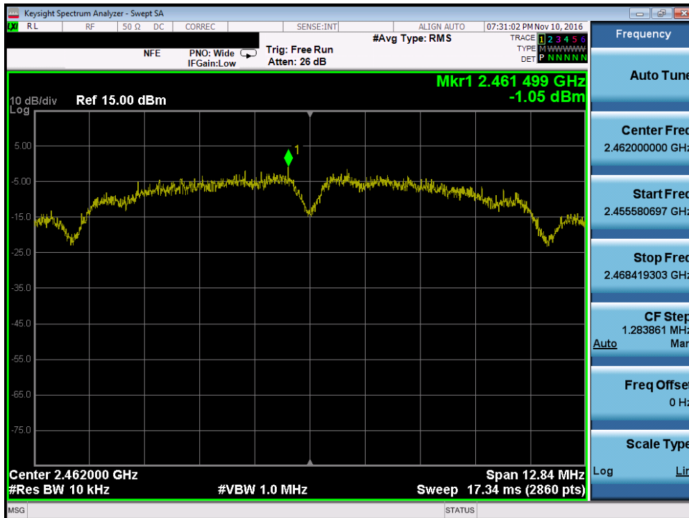
Plot 7-12. Power Spectral Density Plot (802.11b – Ch. 11)
