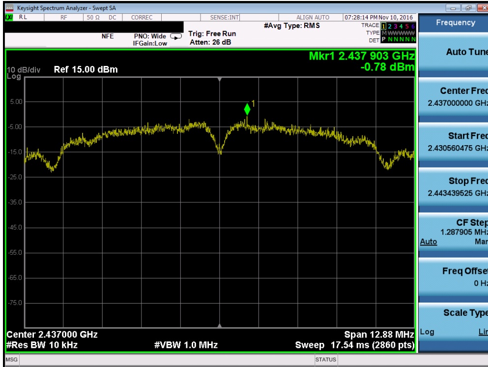
Plot 7-11. Power Spectral Density Plot (802.11b – Ch. 6)
