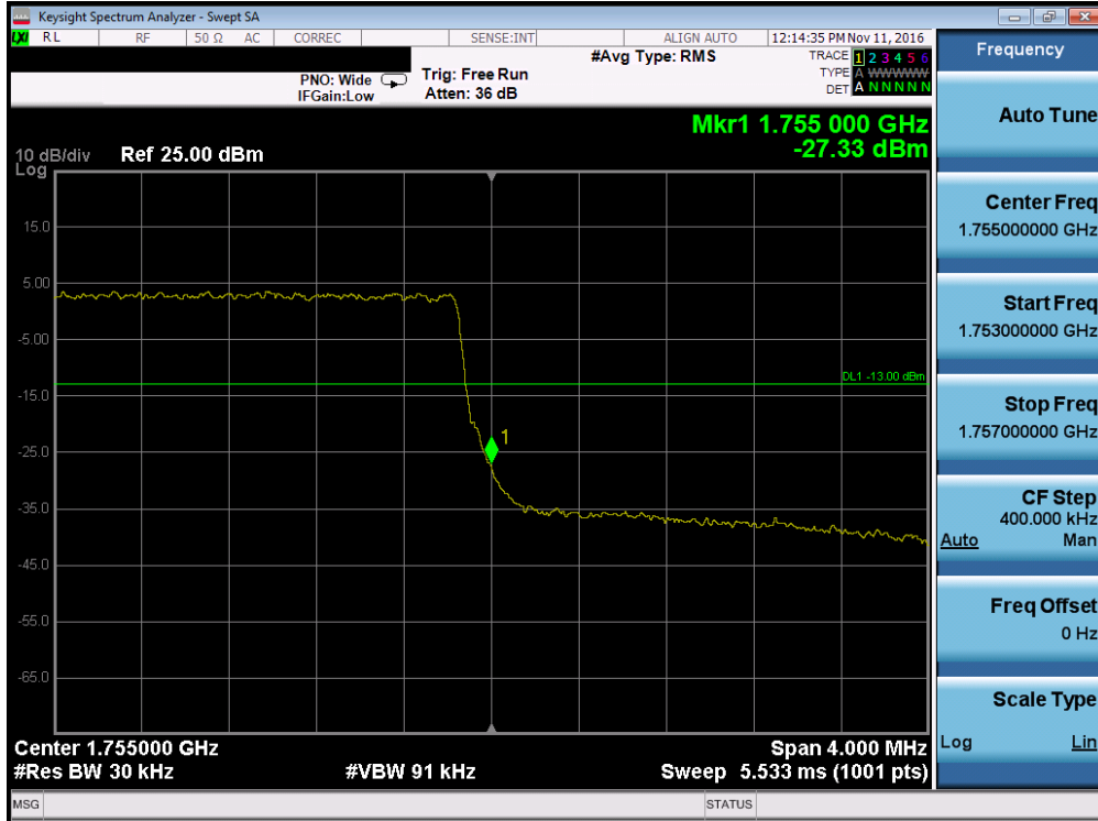
Plot 7-111. Upper Band Edge Plot (Band 4 – 3.0MHz QPSK – RB Size 15)
