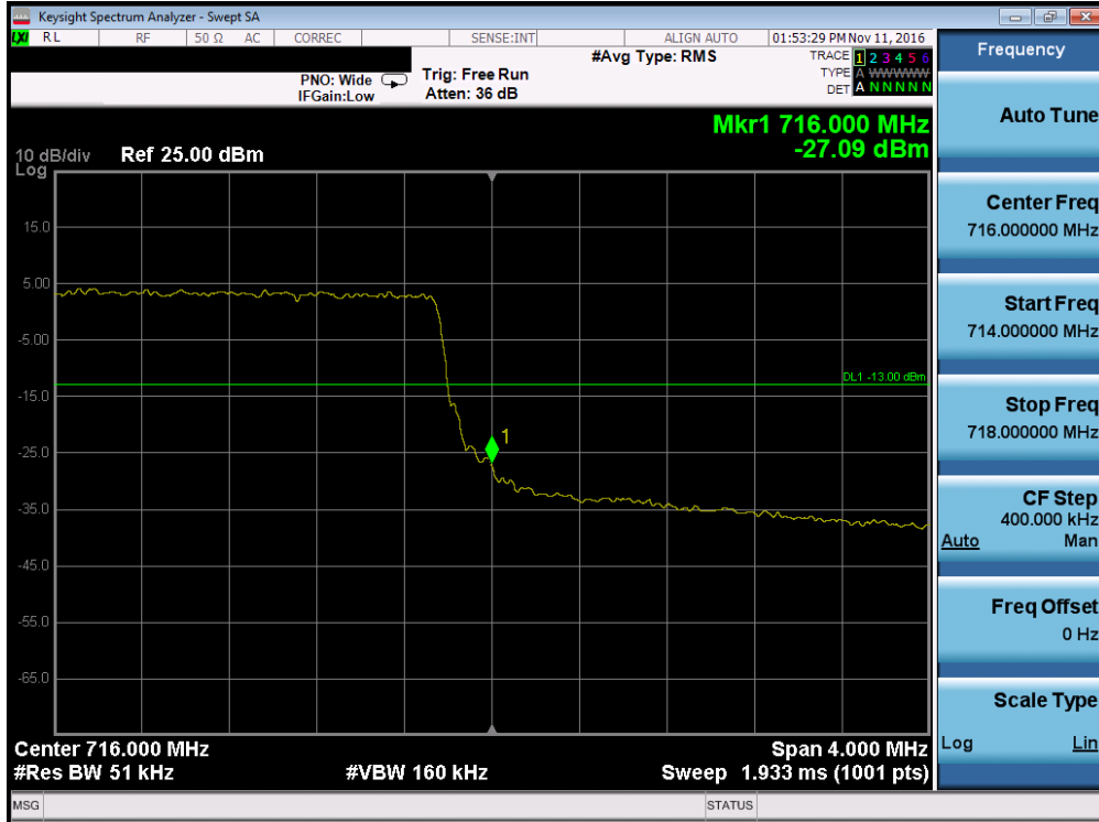
Plot 7-87. Upper Band Edge Plot (Band 12/17 – 5.0MHz QPSK – RB Size 25)
