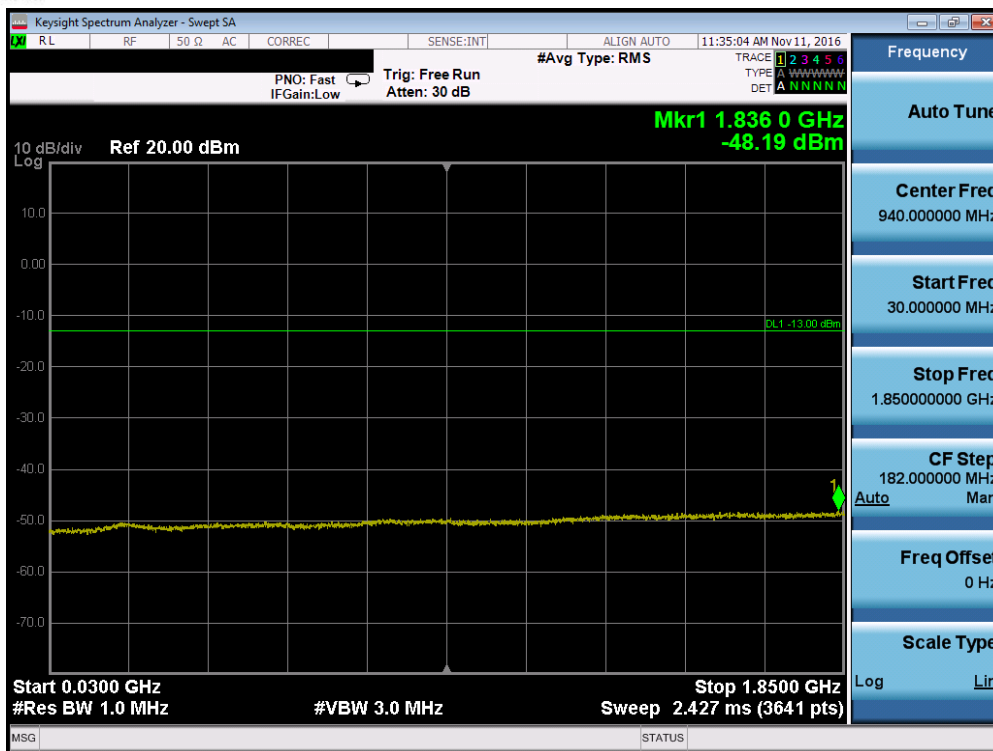
Plot 7-71. Conducted Spurious Plot (Band 2 – 20.0MHz QPSK – RB Size 1, RB Offset 0 – Mid Channel)
