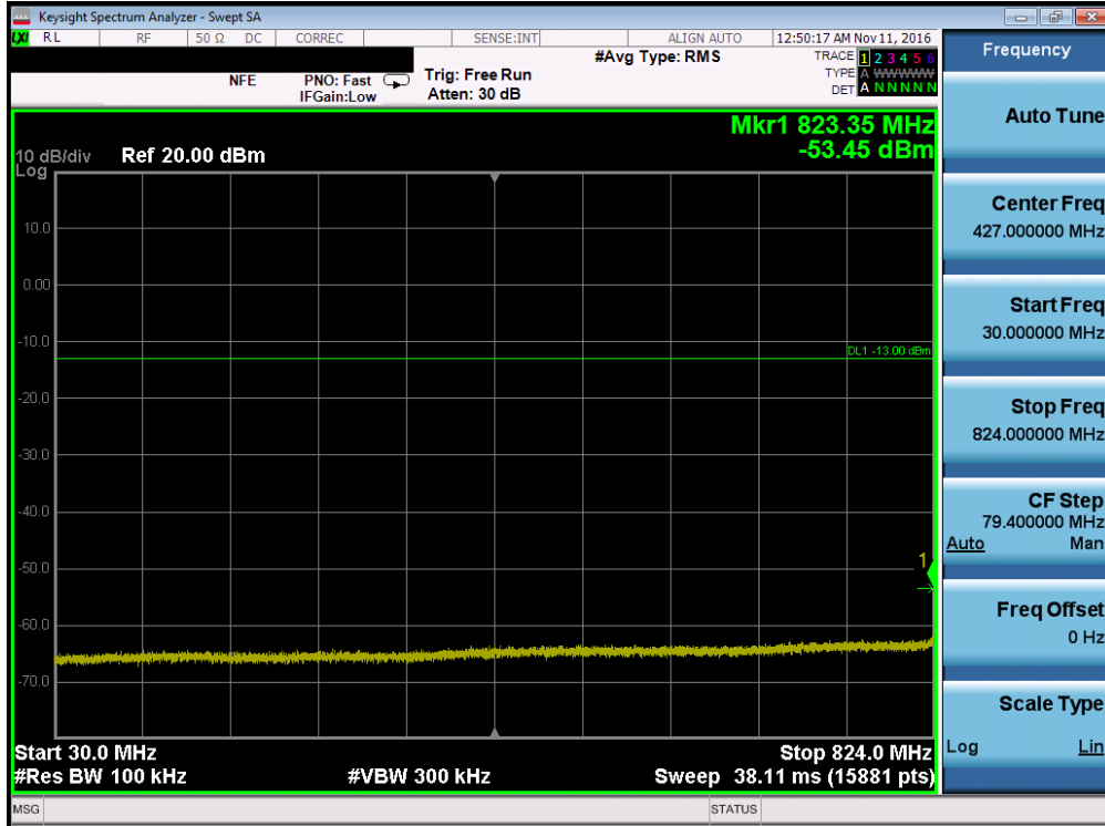
Plot 7-53. Conducted Spurious Plot (Band 5 – 10.0MHz QPSK – RB Size 1, RB Offset 0 – Mid Channel)
