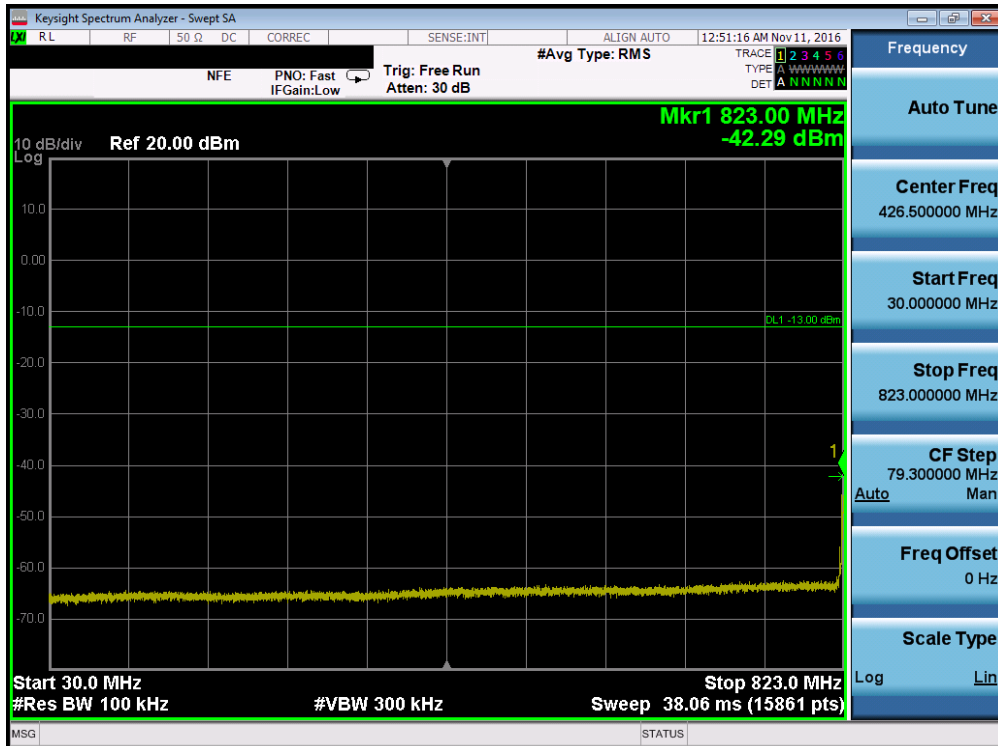
Plot 7-50. Conducted Spurious Plot (Band 5 – 10.0MHz QPSK – RB Size 1, RB Offset 0– Low Channel)
