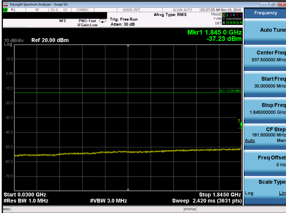
Plot 7-44. Conducted Spurious Plot (PCS WCDMA Mode – Ch. 9262)
