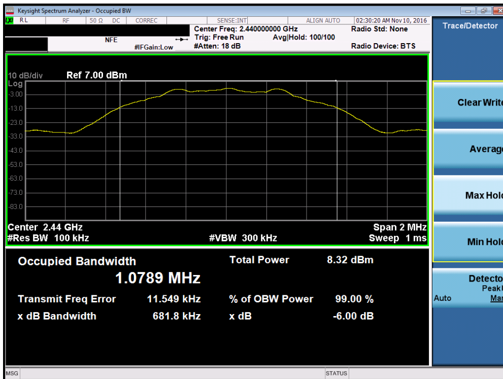
Plot 7-2. 6dB Bandwidth Plot (Bluetooth (LE) – Ch. 19)
