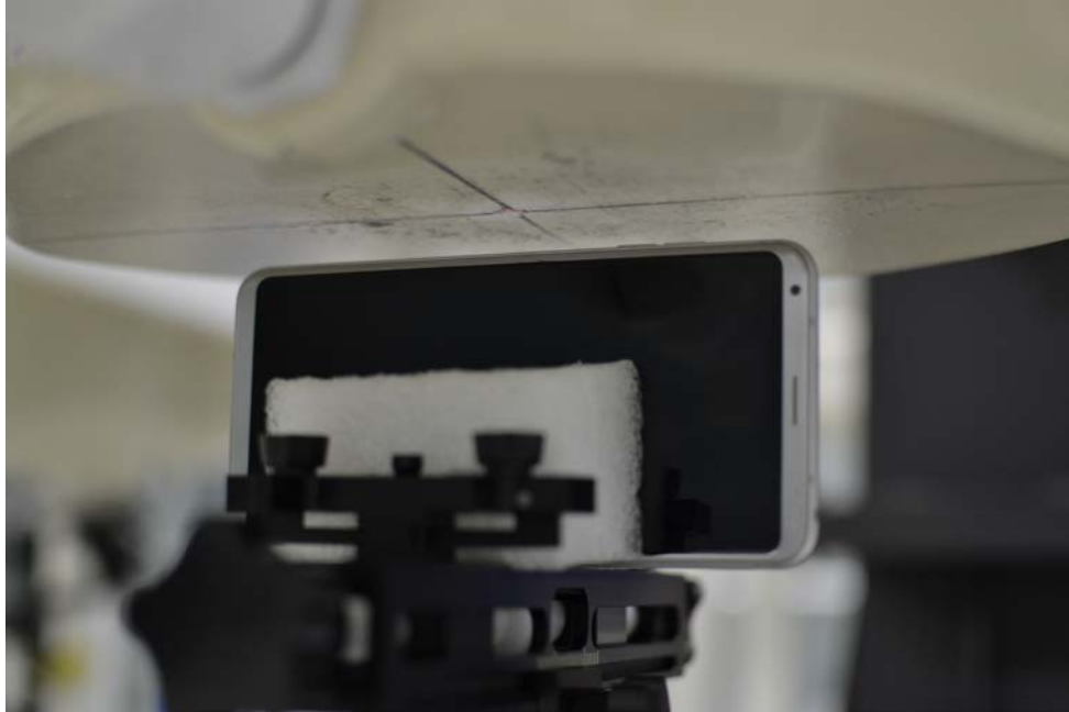
SAR Test Setup Photo 13: Left at 1.0 cm
