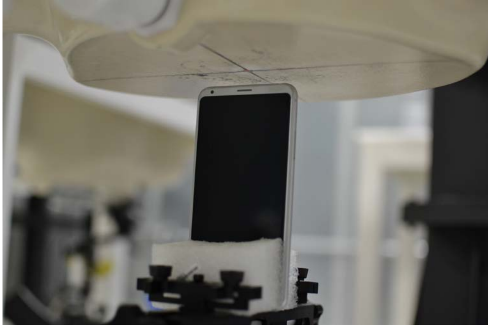
SAR Test Setup Photo 9: Top at 1.0 cm
