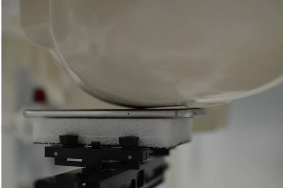
SAR Test Setup Photo 3: Left Cheek
