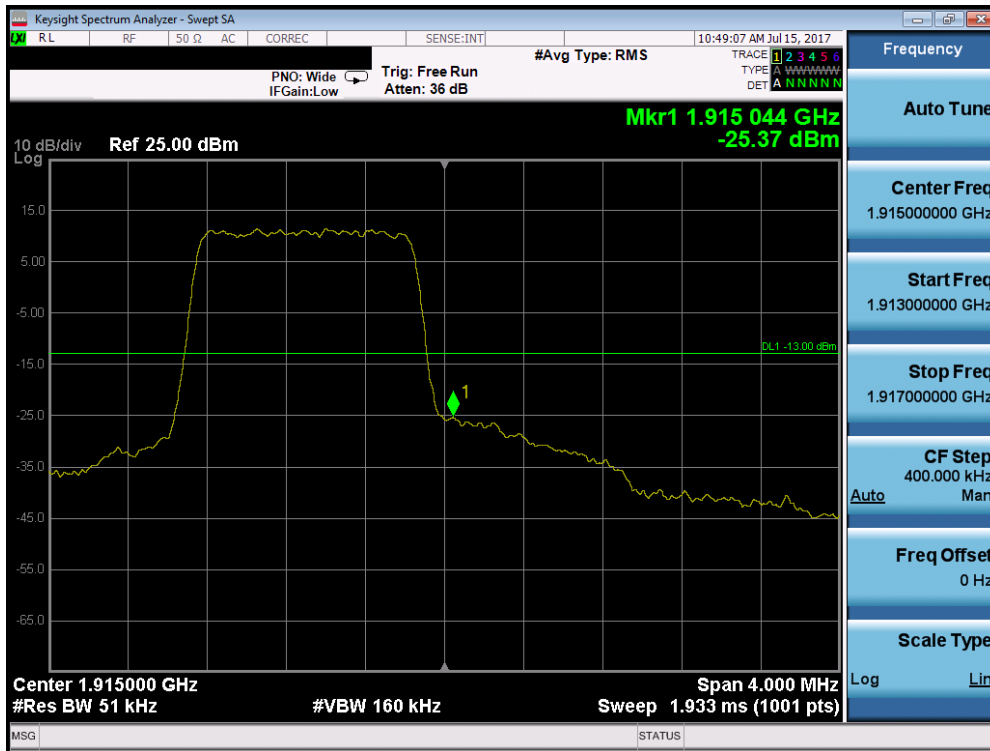
Plot 7-186. Upper Band Edge Plot (Band 25 - 1.4MHz QPSK - RB Size 6)
