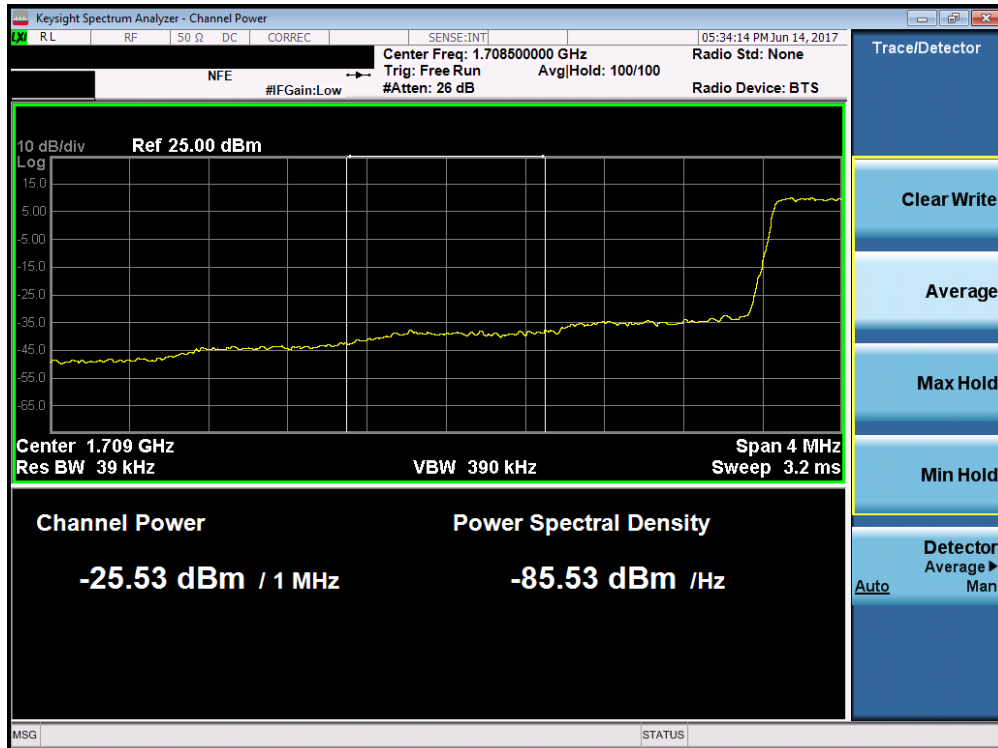
Plot 7-159. Lower Extended Band Edge Plot (Band 4 – 1.4MHz QPSK – RB Size 6)
