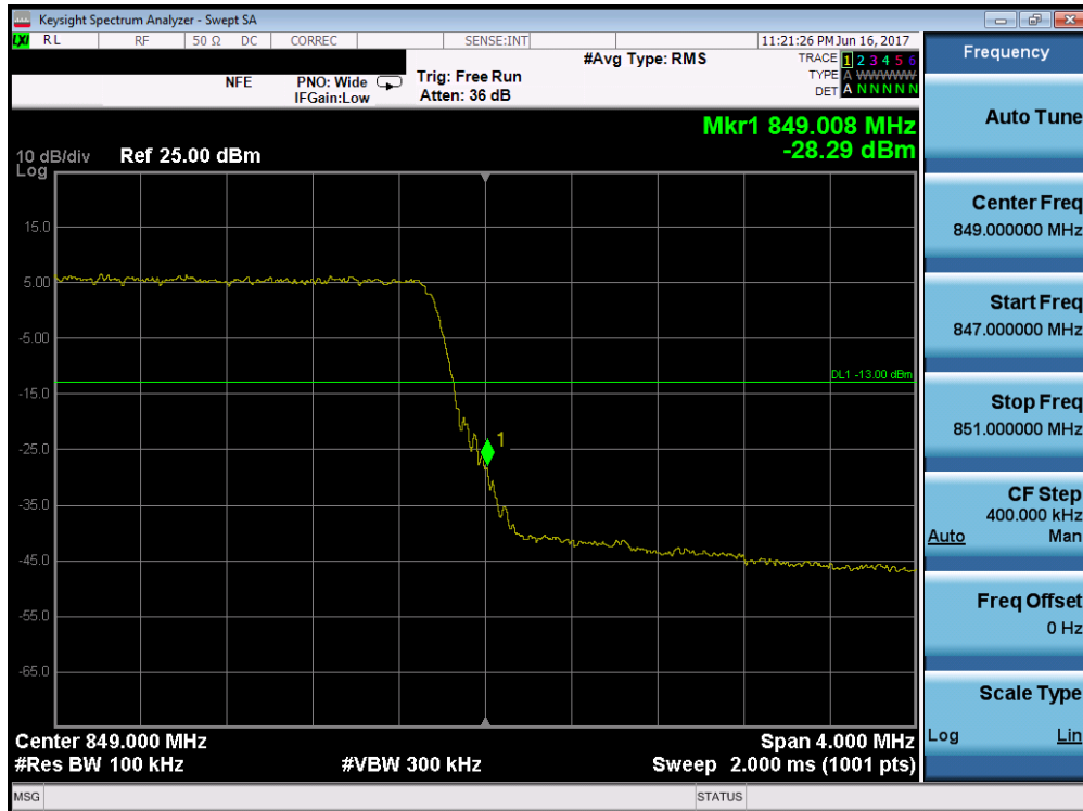
Plot 7-153. Upper Band Edge Plot (Band 5/26 – 5.0MHz QPSK – RB Size 25)
