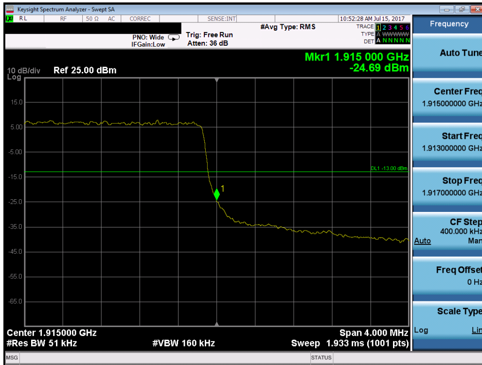
Plot 7-192. Upper Band Edge Plot (Band 25 – 3.0MHz QPSK – RB Size 15)
