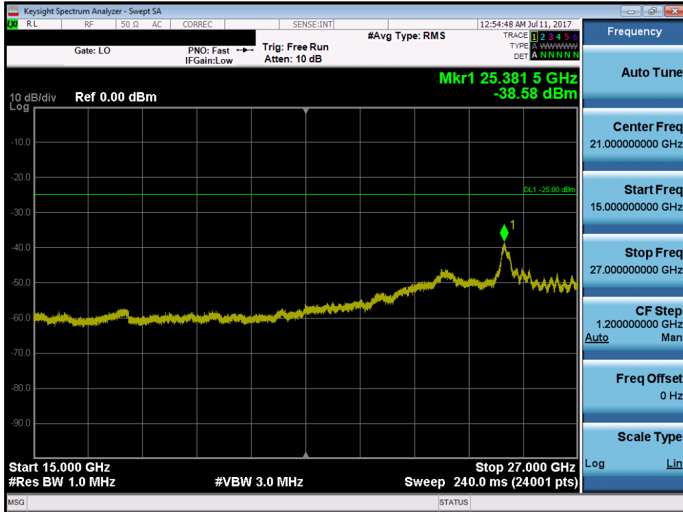
Plot 7-126. Conducted Spurious Plot (Band 41 – 20.0MHz QPSK – RB Size 1, RB Offset 0 – Mid Channel)
