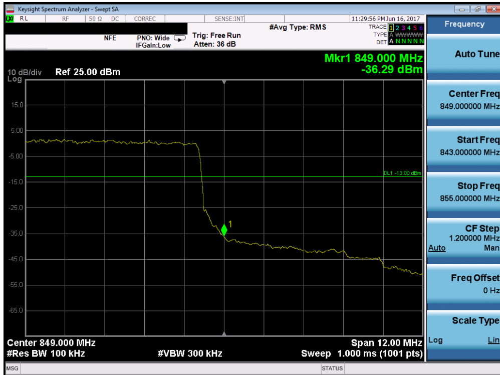
Plot 7-157. Upper Band Edge Plot (Band 5/26 – 15.0MHz QPSK – RB Size 75)
