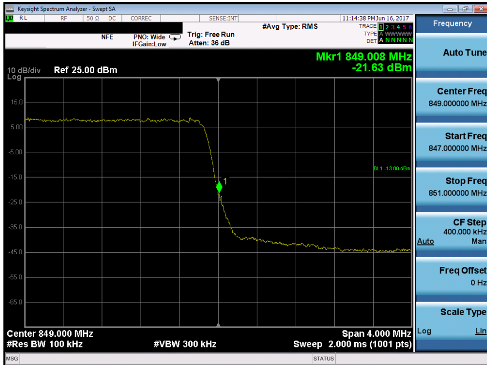
Plot 7-151. Upper Band Edge Plot (Band 5/26 – 3.0MHz QPSK – RB Size 15)
