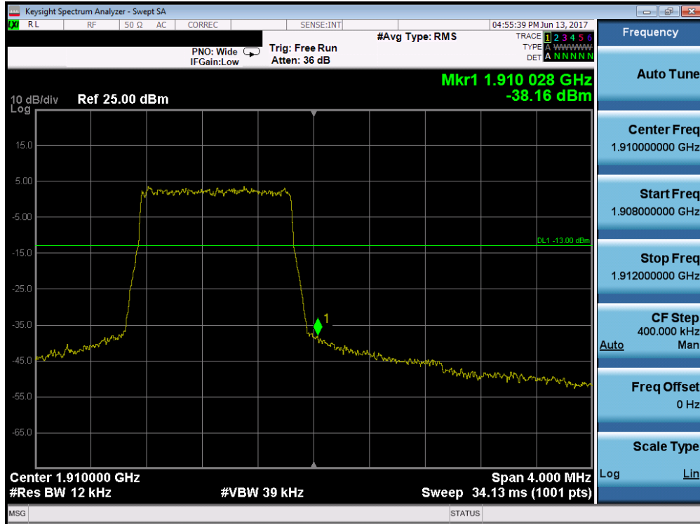
Plot 7-184. Upper Band Edge Plot (Band 2 – 1.4MHz QPSK – RB Size 6)
