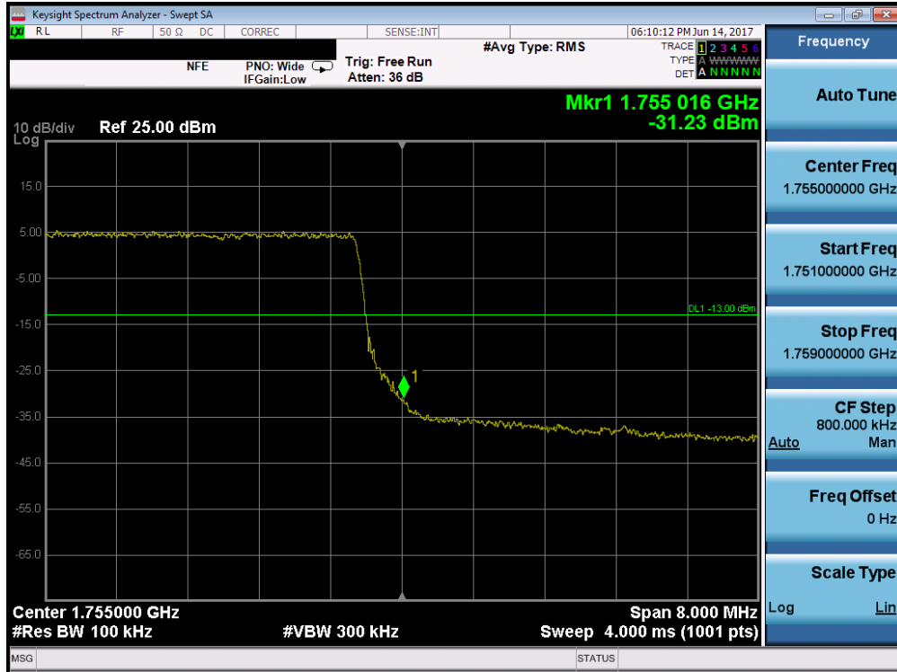
Plot 7-172. Upper Band Edge Plot (Band 4 – 10.0MHz QPSK – RB Size 50)
