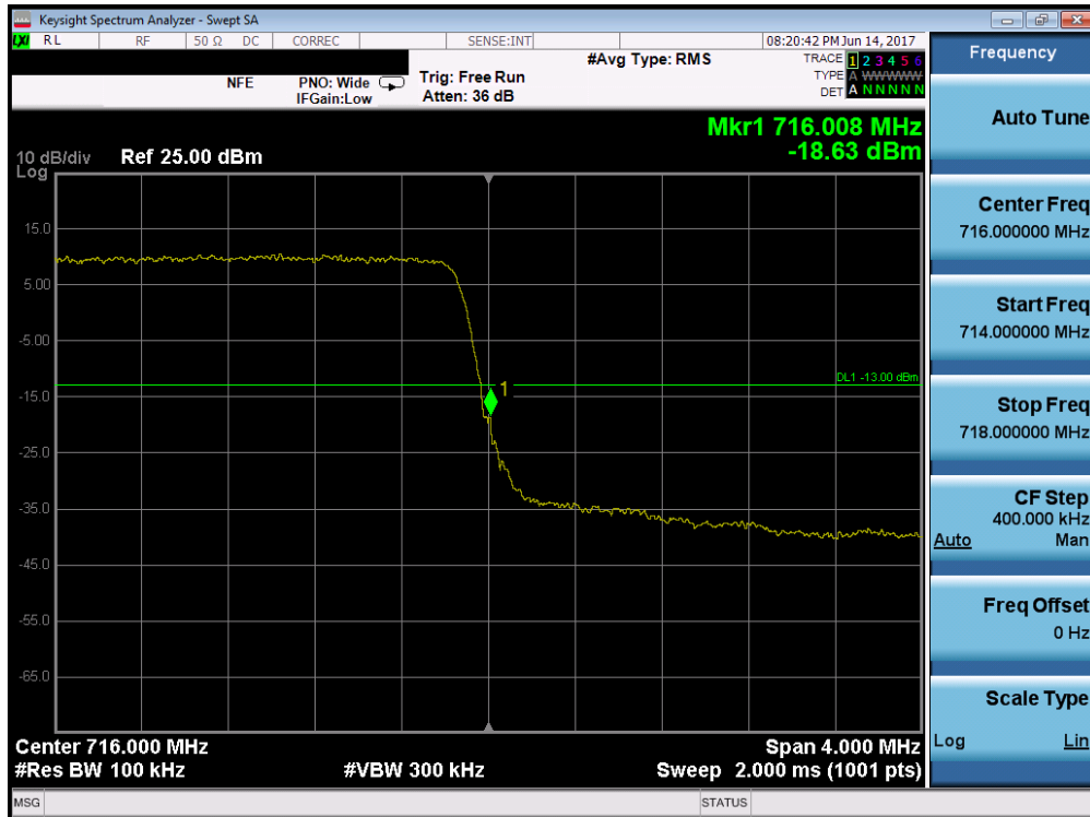
Plot 7-133. Upper Band Edge Plot (Band 12 – 3.0MHz QPSK – RB Size 15)
