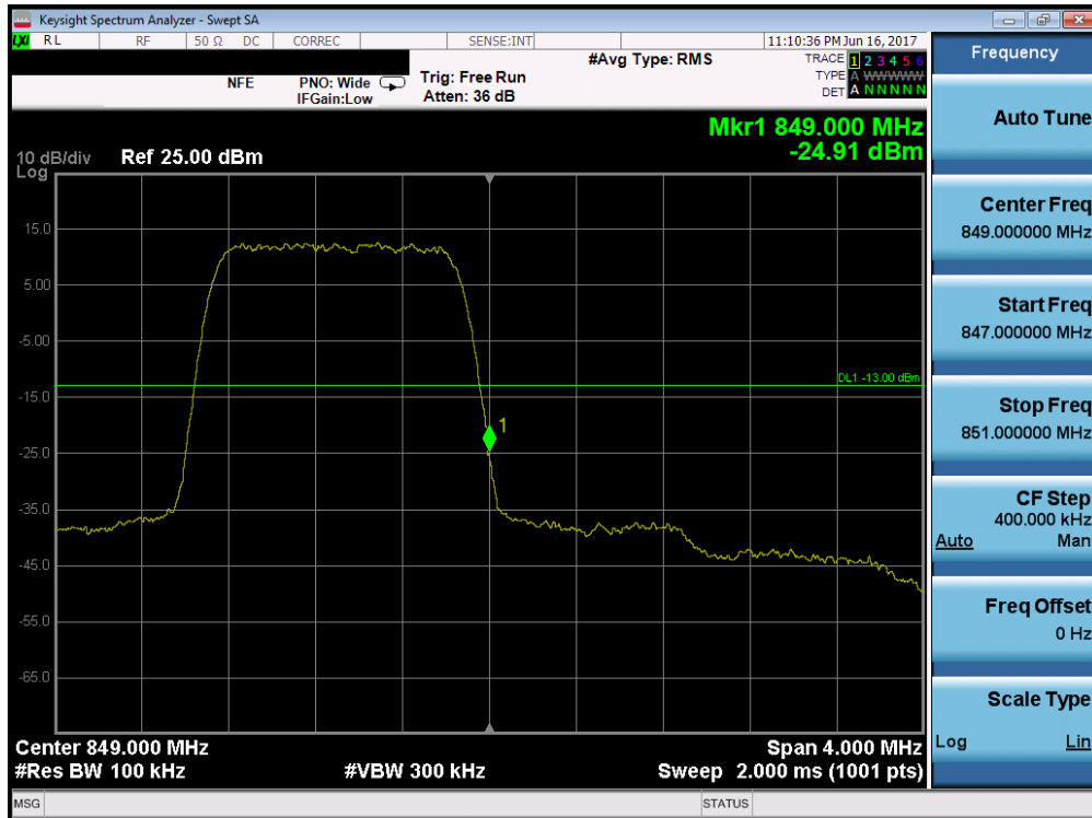
Plot 7-149. Upper Band Edge Plot (Band 5/26 – 1.4MHz QPSK – RB Size 6)
