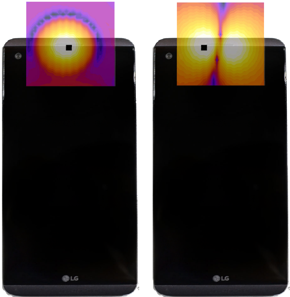
Figure 13-3 T-Coil Scan Overlay Magnetic Field Distributions
