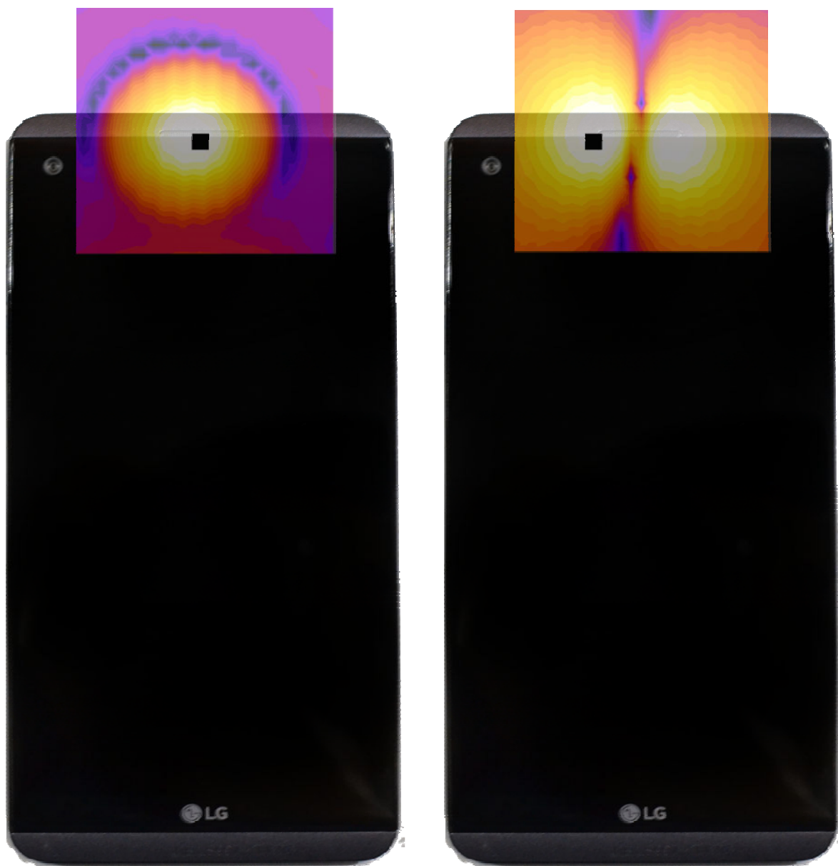
Figure 13-3 T-Coil Scan Overlay Magnetic Field Distributions
