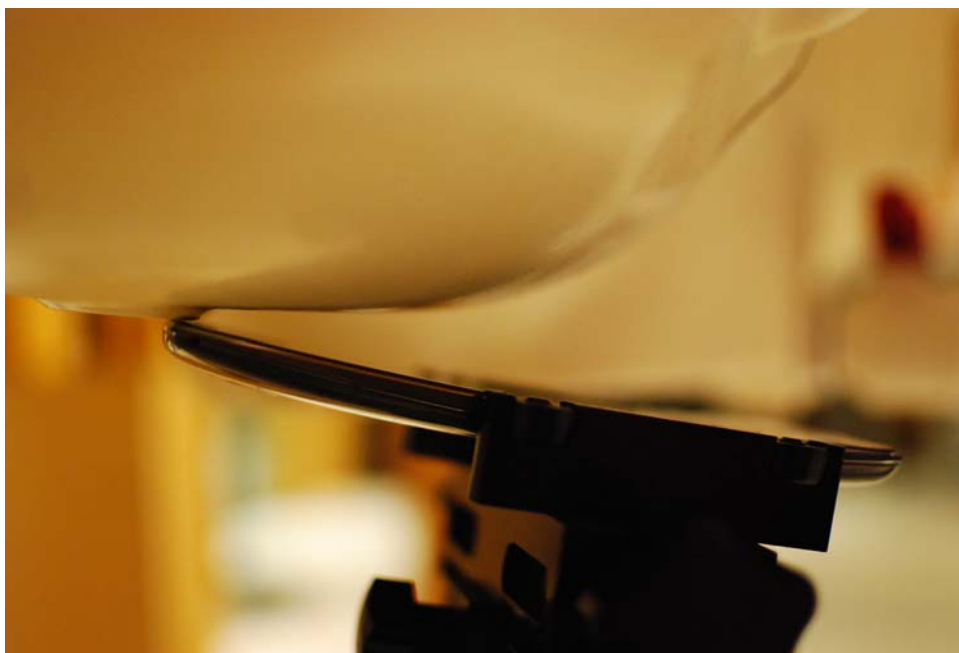
SAR Test Setup Photo 2: Right Tilt
