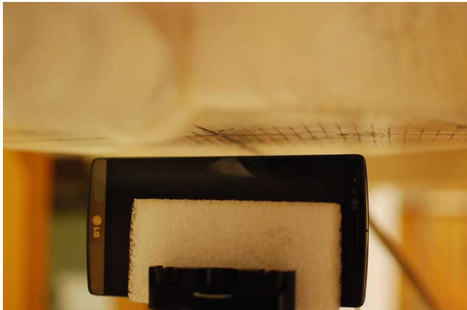
SAR Test Setup Photo 10: Left at 1.0 cm
