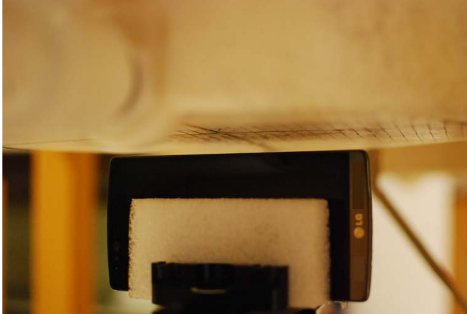
SAR Test Setup Photo 9: Right at 1.0 cm
