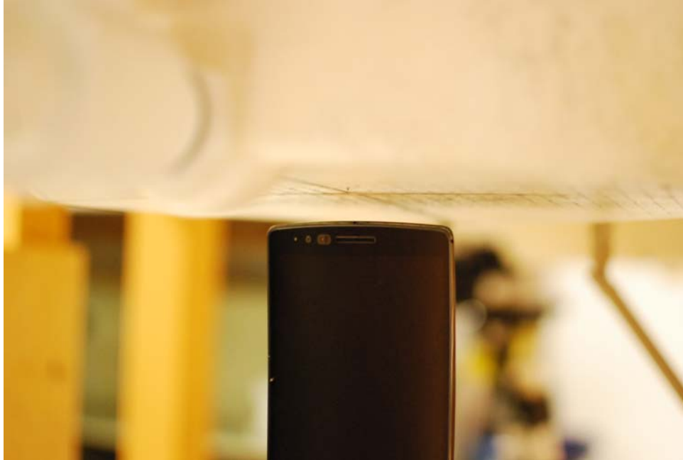
SAR Test Setup Photo 7: Top at 1.0 cm
