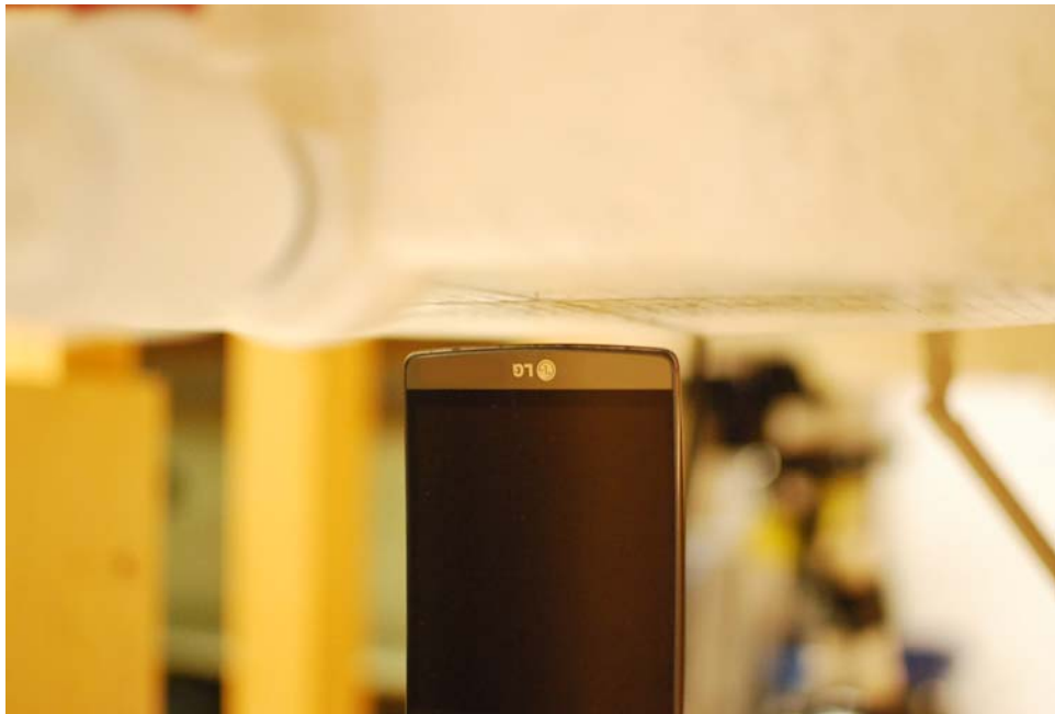
SAR Test Setup Photo 8: Bottom at 1.0 cm
