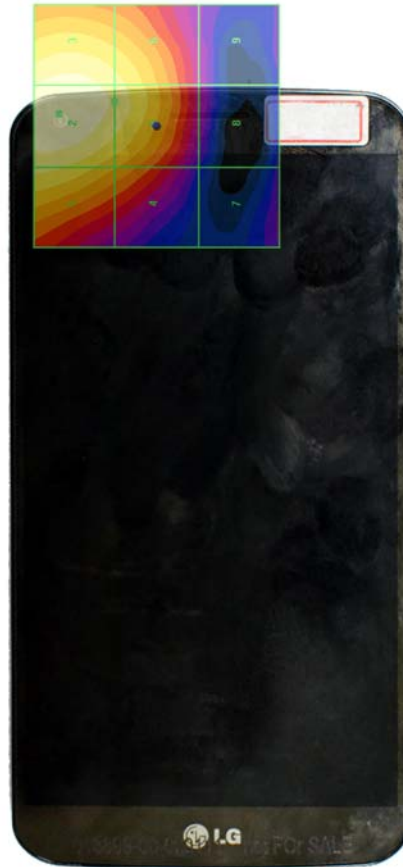
Figure 18-4 E-Field WD Scan overlay (T-Coil Centered Scan pictured)
