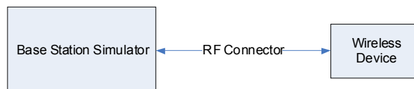
Figure 9-2 Power Measurement Setup
