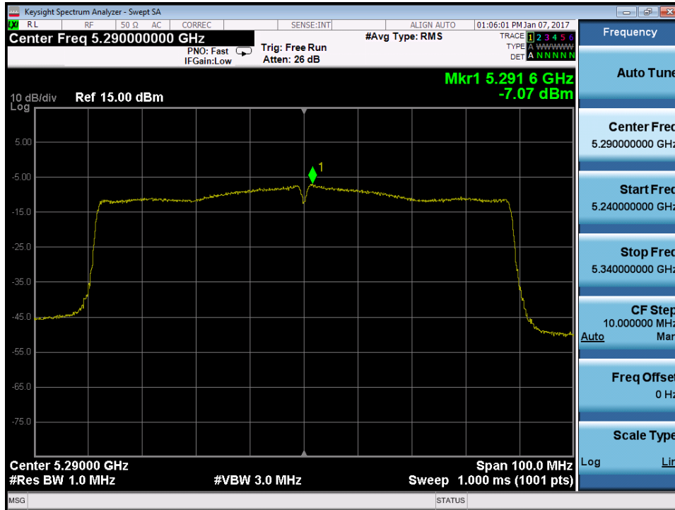
Plot 7-132. Power Spectral Density Plot (80MHz BW 802.11a/n/ac (UNII Band 2A) – Ch. 58)
