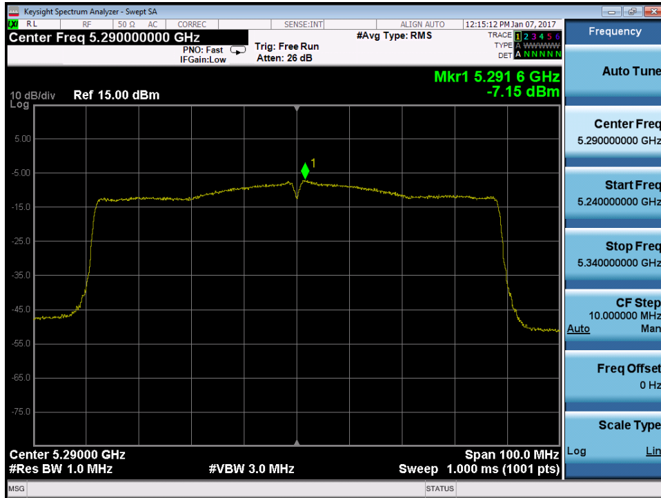
Plot 7-94. Power Spectral Density Plot (80MHz BW 802.11ac (UNII Band 2A) – Ch. 58)
