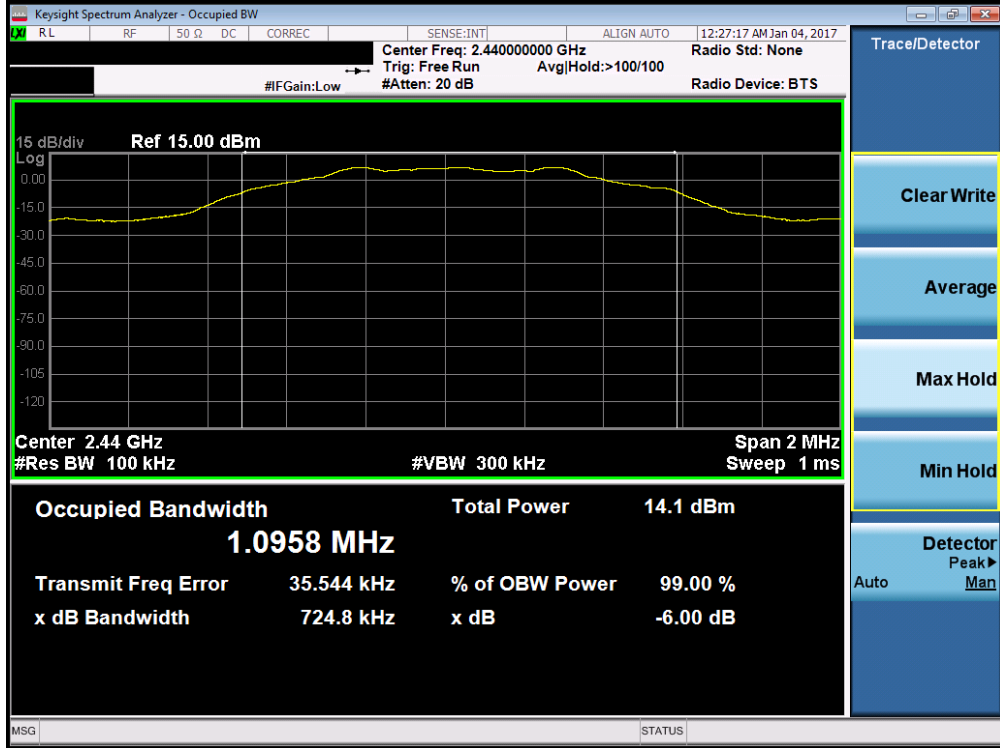
Plot 7-2. 6dB Bandwidth Plot (Bluetooth (LE) – Ch. 19)
