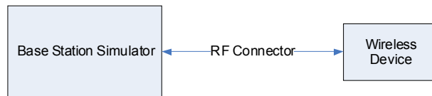
Figure 9-2 Power Measurement Setup
