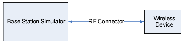
Figure 9-4 Power Measurement Setup
