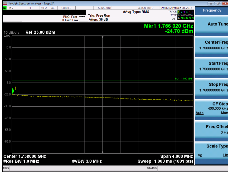
Plot 7-158. Upper Extended Band Edge Plot (Band 4 – 15.0MHz QPSK – RB Size 75)
