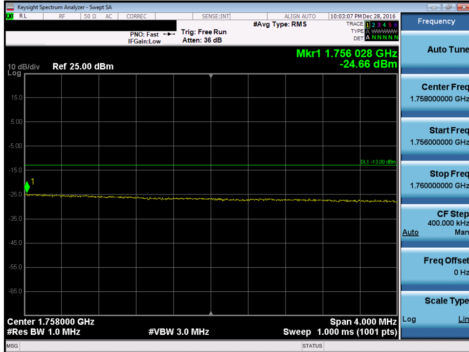
Plot 7-162. Upper Extended Band Edge Plot (Band 4 – 20.0MHz QPSK – RB Size 100)
