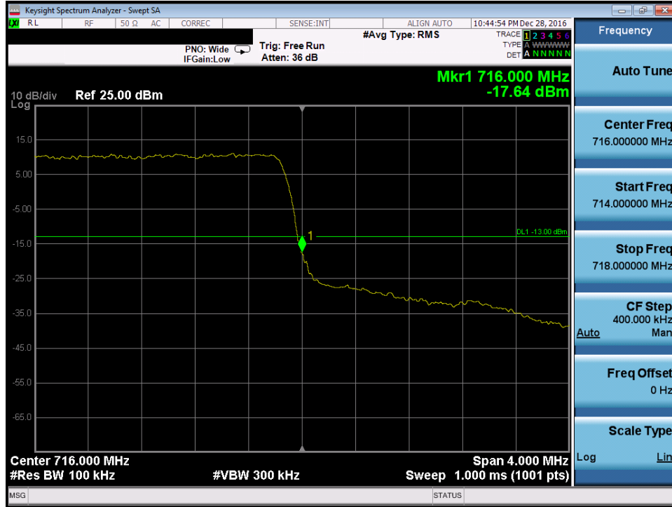
Plot 7-124. Upper Band Edge Plot (Band 12 – 3.0MHz QPSK – RB Size 15)
