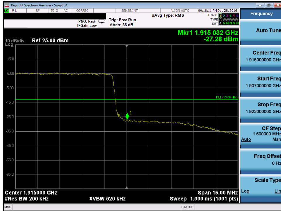
Plot 7-185. Upper Band Edge Plot (Band 25/2 – 20.0MHz QPSK – RB Size 100)
