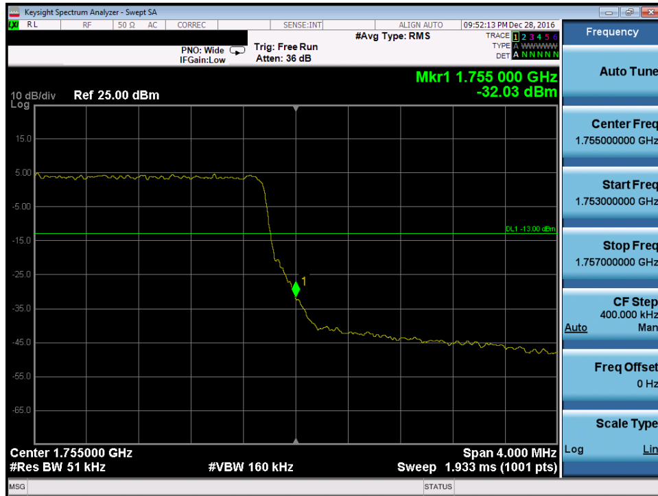
Plot 7-149. Upper Band Edge Plot (Band 4 – 5.0MHz QPSK – RB Size 25)
