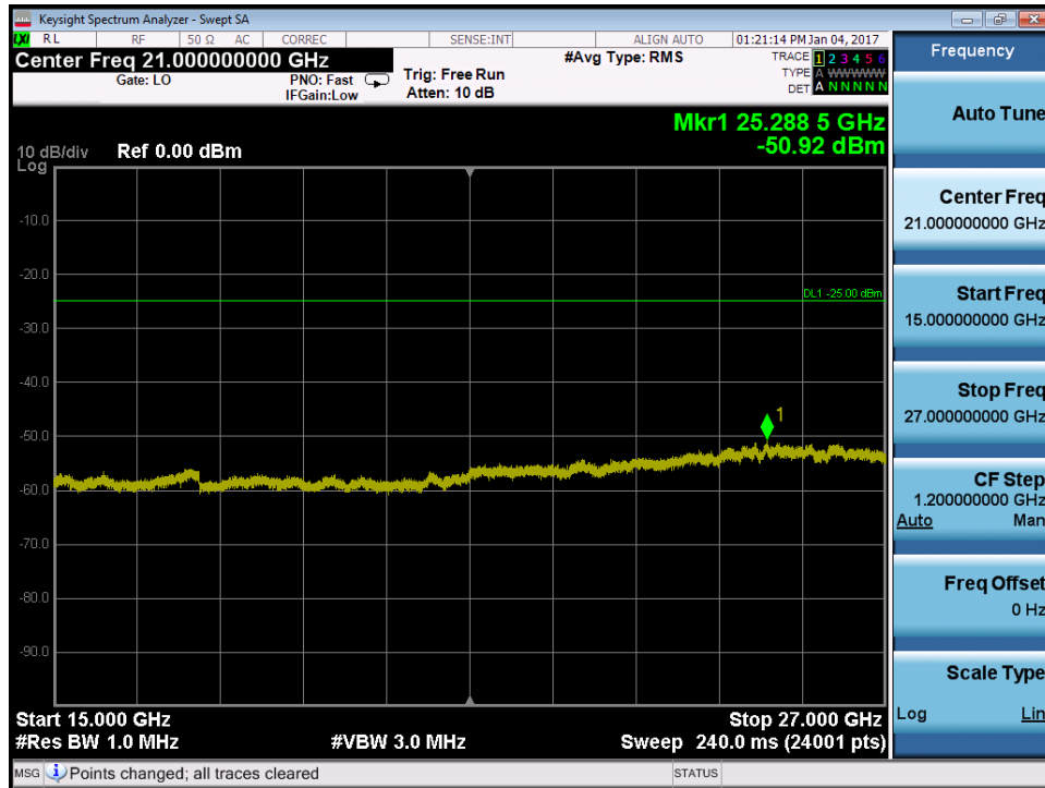
Plot 7-117. Conducted Spurious Plot (Band 41 – 5.0MHz QPSK – RB Size 1, RB Offset 0 – Mid Channel)
