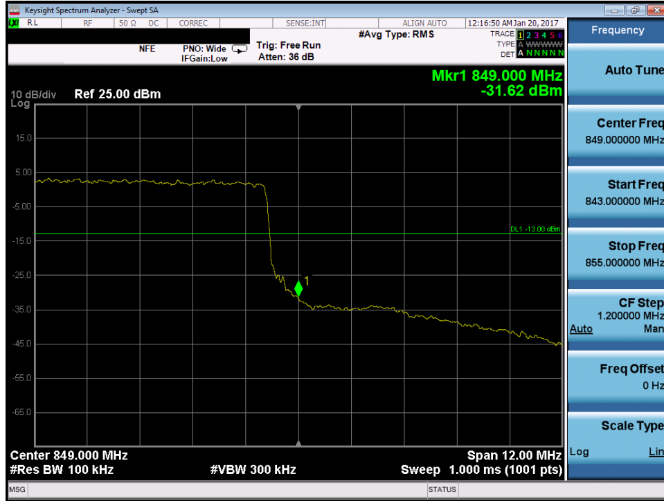
Plot 7-138. Upper Band Edge Plot (Band 26/5 – 15.0MHz QPSK – RB Size 75)
