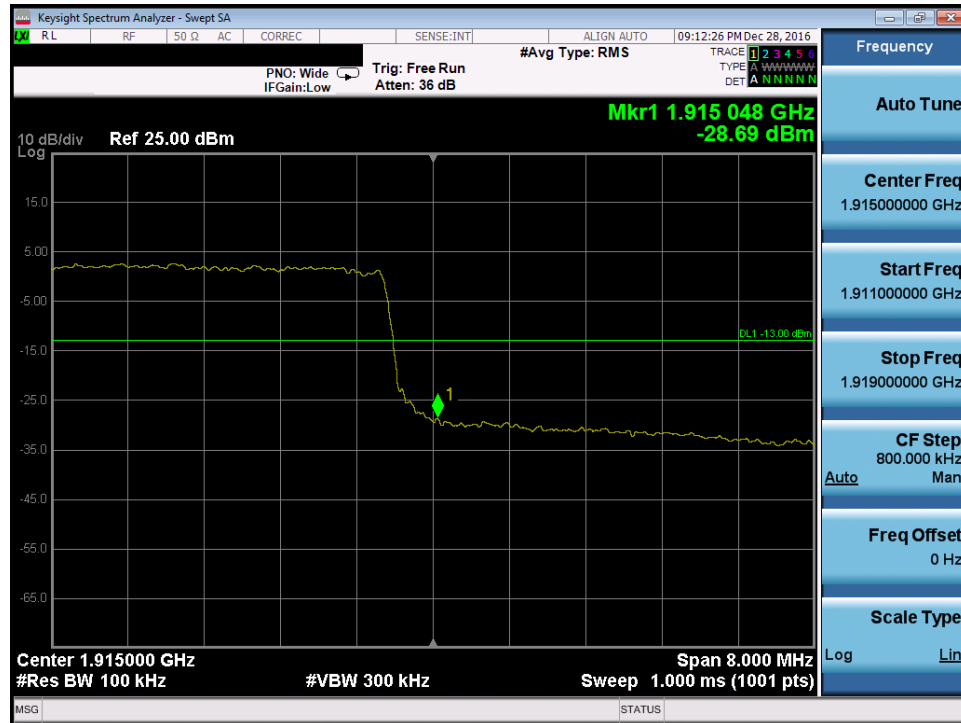
Plot 7-177. Upper Band Edge Plot (Band 25/2 – 10.0MHz QPSK – RB Size 50)
