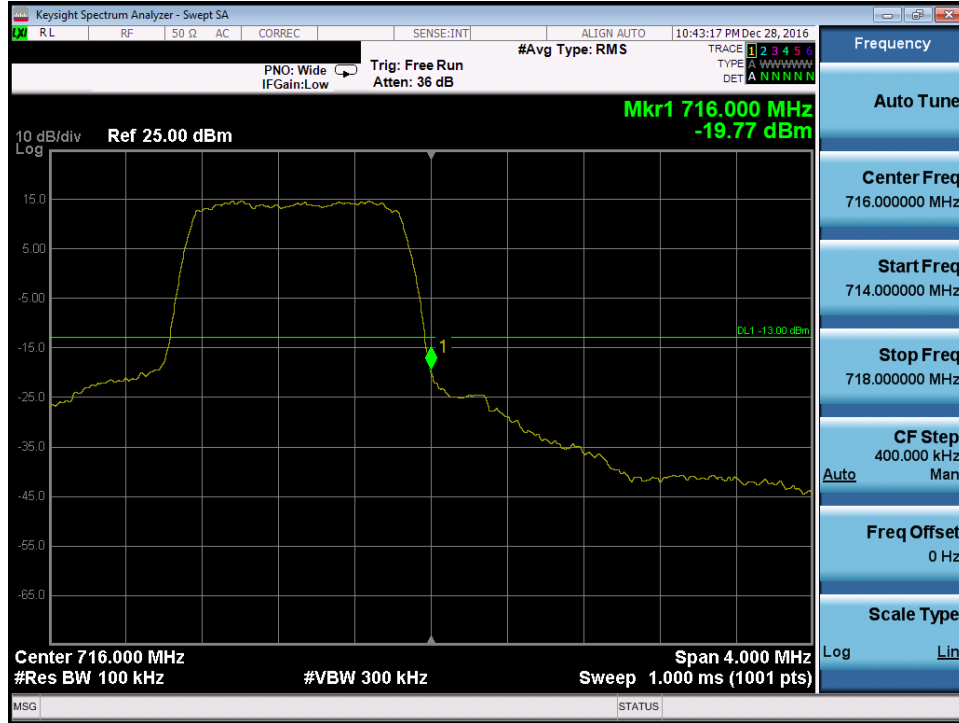
Plot 7-122. Upper Band Edge Plot (Band 12 – 1.4MHz QPSK – RB Size 6)
