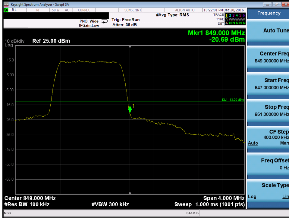
Plot 7-130. Upper Band Edge Plot (Band 26/5 – 1.4MHz QPSK – RB Size 6)
