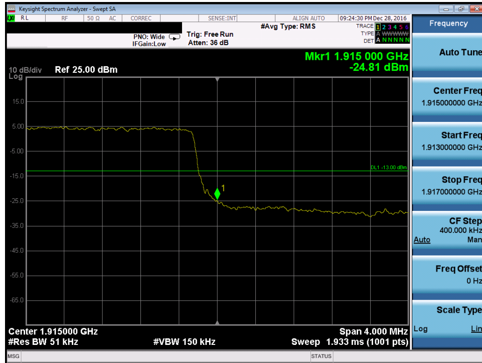
Plot 7-173. Upper Band Edge Plot (Band 25/2 – 5.0MHz QPSK – RB Size 25)
