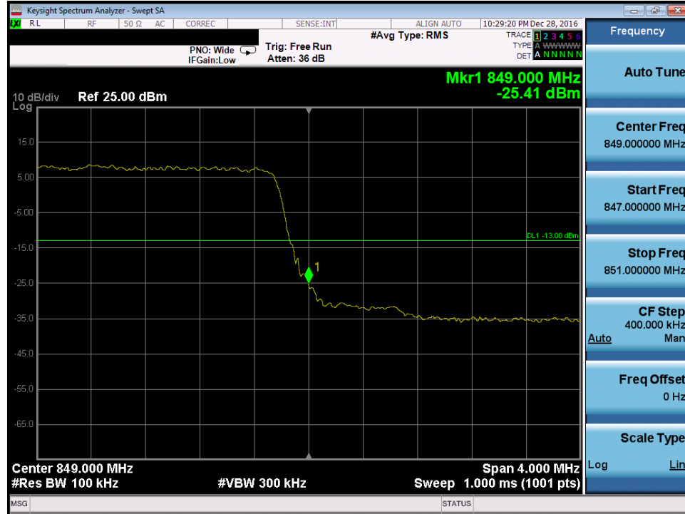
Plot 7-134. Upper Band Edge Plot (Band 26/5 – 5.0MHz QPSK – RB Size 25)
