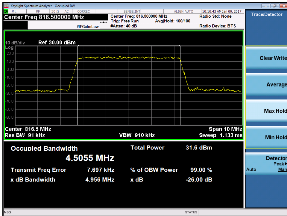
Plot 7-10. Occupied Bandwidth Plot LTE B26 (5MHz 16-QAM – RB Size 25– Low Channel)
