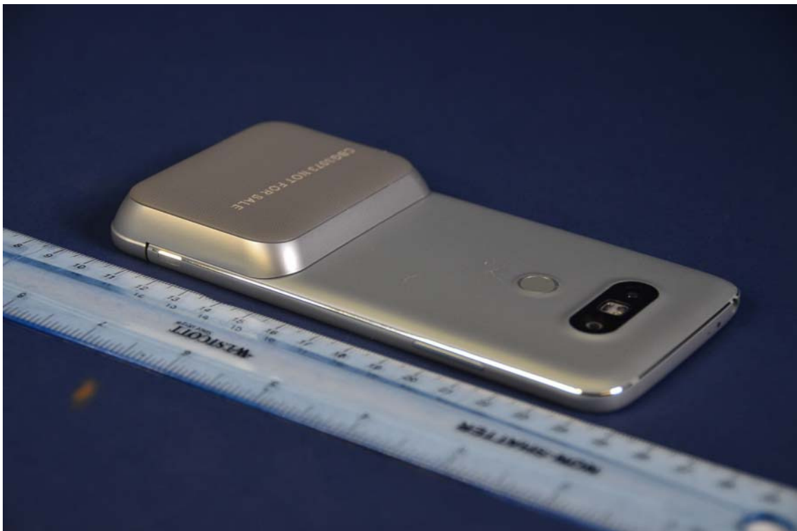
Camera Module Installed
