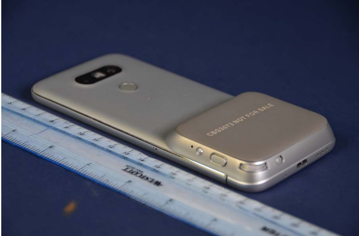
Camera Module Installed
