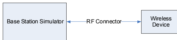
Figure 9-3 Power Measurement Setup
