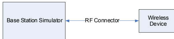
Figure 9-1 Power Measurement Setup
