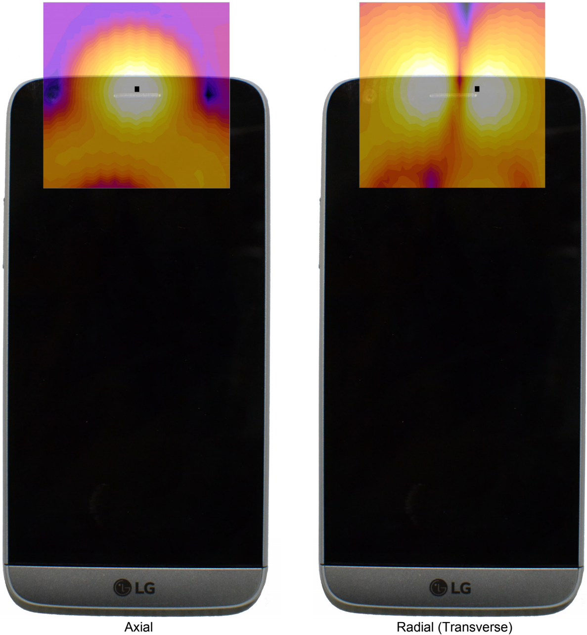
Figure 14-5 T-Coil Scan Overlay Magnetic Field Distributions
