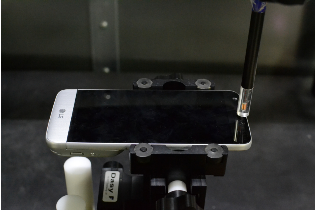
Figure 14-3 Test Setup for Wireless Device – Camera Module Accessory
