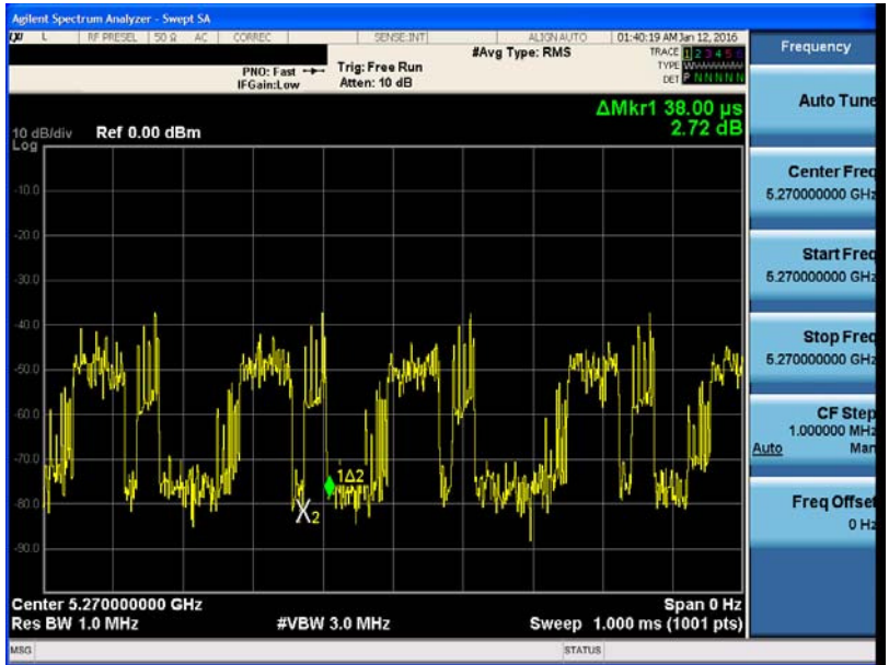
Figure 5-1. Band 2A Pulse Width
