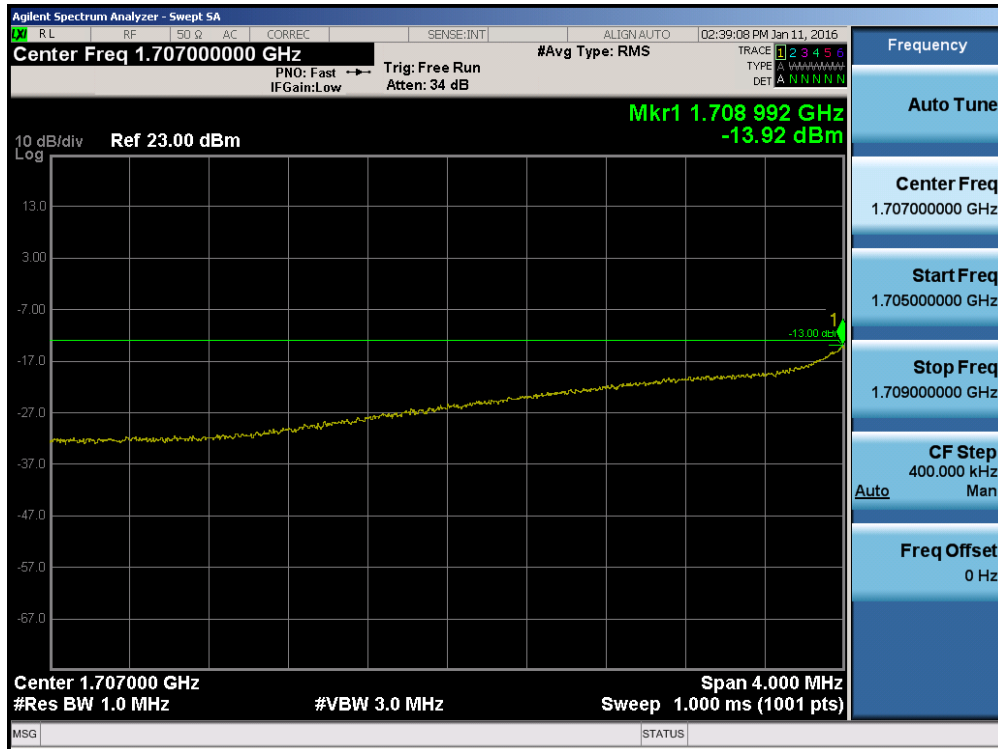
Plot 7-90. 4MHz Span Plot (AWS WCDMA Mode – Ch. 1312)
