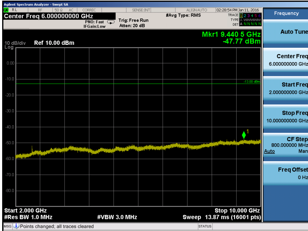
Plot 7-54. Conducted Spurious Plot (Cellular WCDMA Mode – Ch. 4233)
