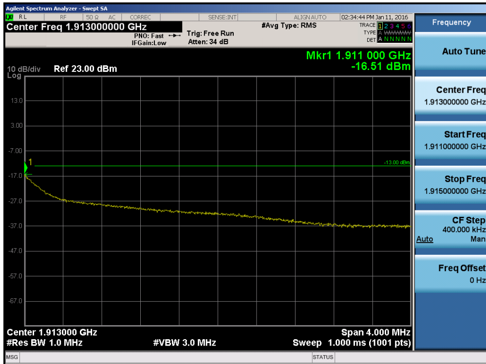
Plot 7-96. 4MHz Span Plot (PCS WCDMA Mode – Ch. 9538)
