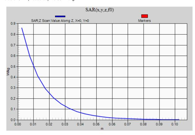
Frequency: 5200 MHz; Duty Cycle: 1:1; Room Ambient Temperature: 24.0°C; Liquid Temperature: 23.0°C Medium parameters used: f = 5200 MHz;  $\sigma$  = 4.626 S/m;  $\epsilon_r$  = 36.513;  $\rho$  = 1000 kg/m<sup>3</sup> DASY5 Configuration:
