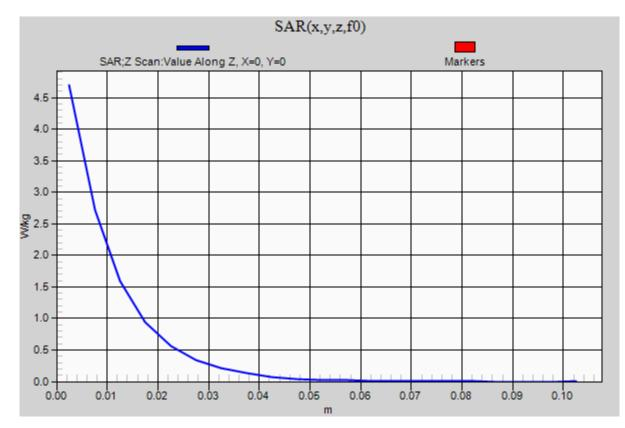
Frequency: 835 MHz; Duty Cycle: 1:1; Room Ambient Temperature: 24.0°C; Liquid Temperature: 23.0°C Medium parameters used: f = 835 MHz;  $\sigma$  = 1.011 S/m;  $\epsilon_r$  = 54.144;  $\rho$  = 1000 kg/m<sup>3</sup> DASY5 Configuration:
