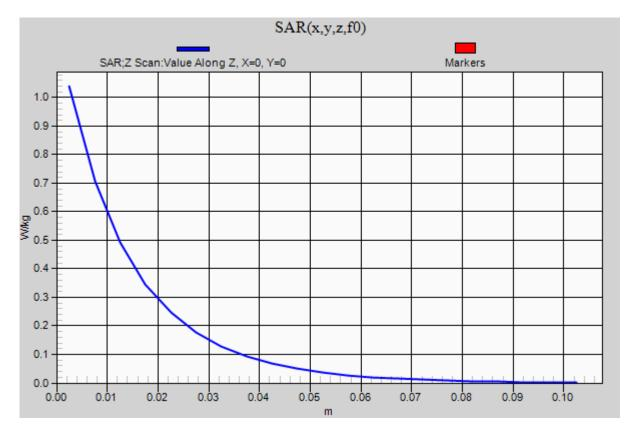
Frequency: 1750 MHz; Duty Cycle: 1:1; Room Ambient Temperature: 24.0°C; Liquid Temperature: 23.0°C Medium parameters used: f = 1750 MHz;  $\sigma$  = 1.526 S/m;  $\epsilon_r$  = 54.92;  $\rho$  = 1000 kg/m<sup>3</sup> DASY5 Configuration:
