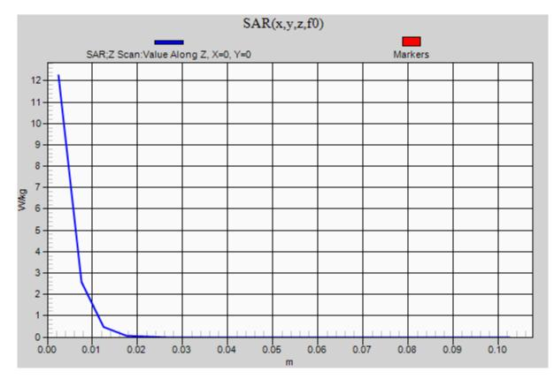
Frequency: 1900 MHz; Duty Cycle: 1:1; Room Ambient Temperature: 24.0°C; Liquid Temperature: 23.0°C Medium parameters used: f = 1900 MHz;  $\sigma$  = 1.518 S/m;  $\epsilon_r$  = 53.381;  $\rho$  = 1000 kg/m<sup>3</sup> DASY5 Configuration:
