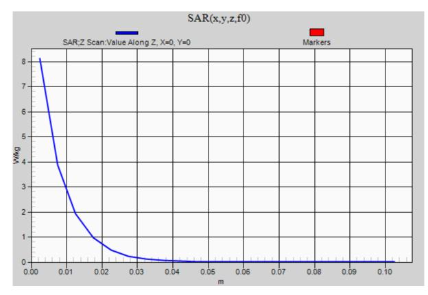
Frequency: 2450 MHz; Duty Cycle: 1:1; Room Ambient Temperature: 24.0°C; Liquid Temperature: 23.0°C Medium parameters used: f = 2450 MHz;  $\sigma$  = 1.884 S/m;  $\epsilon_r$  = 39.46;  $\rho$  = 1000 kg/m<sup>3</sup> DASY5 Configuration:
