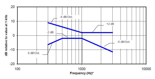
NOTE—The frequency response is between 300 Hz and 3000 Hz.
