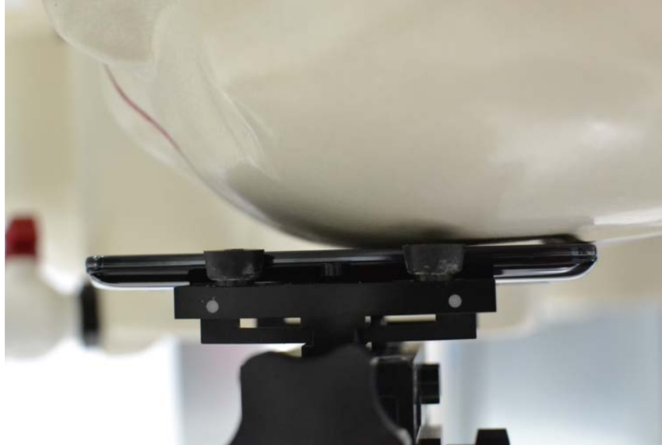
SAR Test Setup Photo 3: Left Cheek
