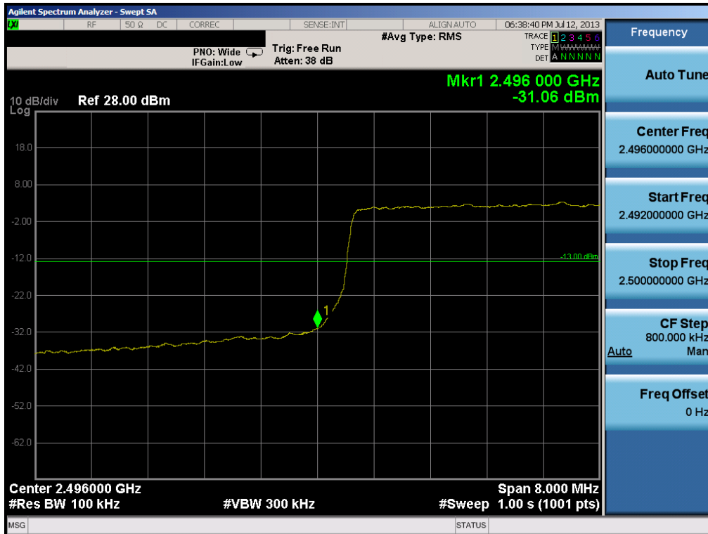
Plot 9-4. Low Channel Band Edge Plot (10.0MHz QPSK – RB Size 50)
