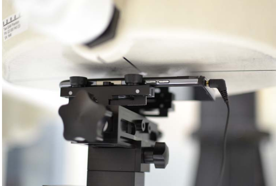
SAR Test Setup Photo 11: Body-worn back side at 1.0 cm
