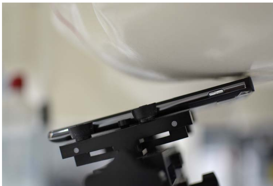
SAR Test Setup Photo 4: Left Tilt
