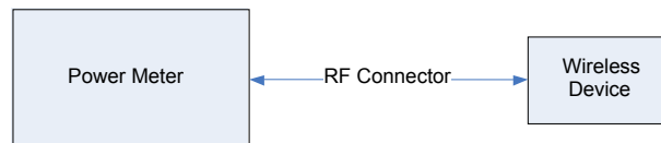
Figure 10-3 Power Measurement Setup
