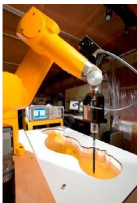
Figure 4-1 SAR Measurement System
