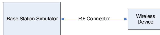
Figure 10-2 Power Measurement Setup
