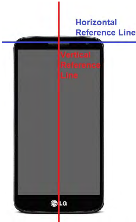
SAR Test Setup Photo 11: Vertical and Horizontal Reference Lines
