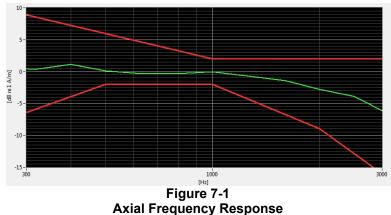
Note: User T-coil Mode (**Settings->Call Settings->Hearing aids**) was set to ON for Frequency Response compliance. This frequency response represents the worst-case ABM2 test configuration according to Table 7-3.
