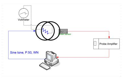
Figure 5-1 Validation Setup with Helmholtz Coil
