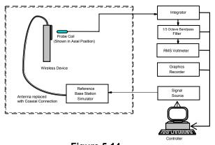
Figure 5-14 **Audio Magnetic Field Test Setup**
