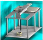
Figure 5-3 RF Near-Field Scanner
