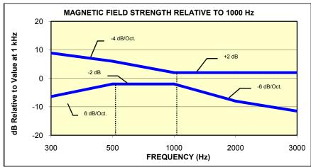
Figure 4-1 Magnetic field frequency response for Wireless Devices with an axial field ≤-15 dB (A/m) at 1 kHz
