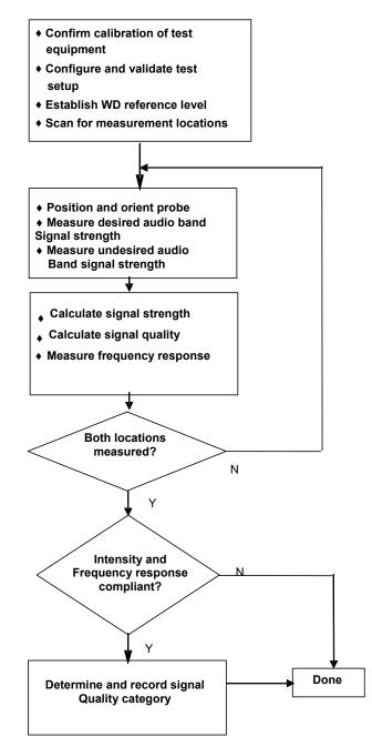
Figure 5-16 C63.19 T-Coil Signal Test Process
