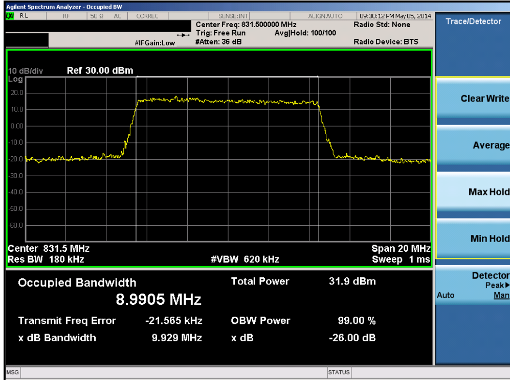
Plot 6-7. Occupied Bandwidth Plot (Band 26 – 10.0MHz QPSK – RB Size 50)
