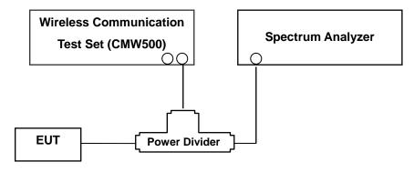
(Configuration of conducted Emission measurement)
