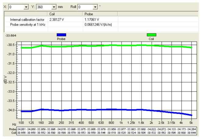
Figure 3: Frequency Response measured in AMCC
