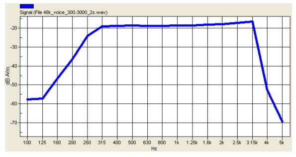
Figure 8: Broadband signal spectrum
