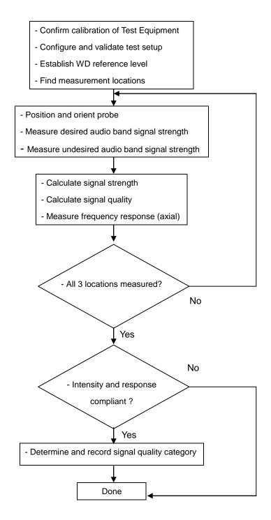
Figure 6: T-Coil measurement flowchart
