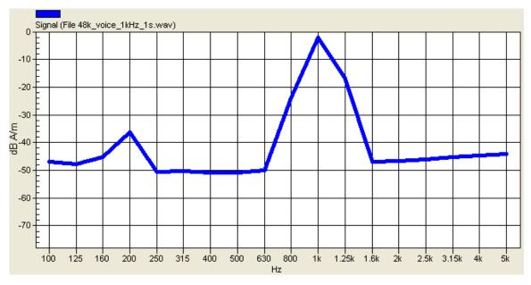
Figure 7: 1 KHz Voice signal spectrum
