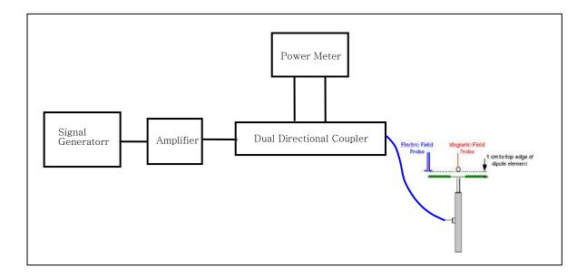
Figure 6. Dipole Validation SET-UP
