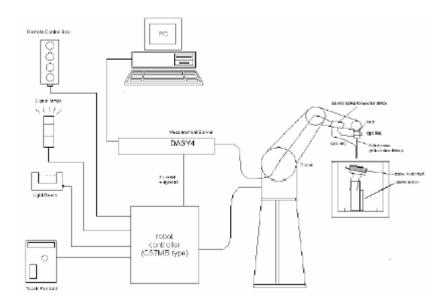
Figure 1. HAC Test Measurement Set-up
