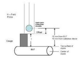
Figure 4. Gauge Block with E-Field Probe
