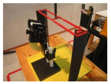
Figure 2. HAC Phantom & Device Holder
