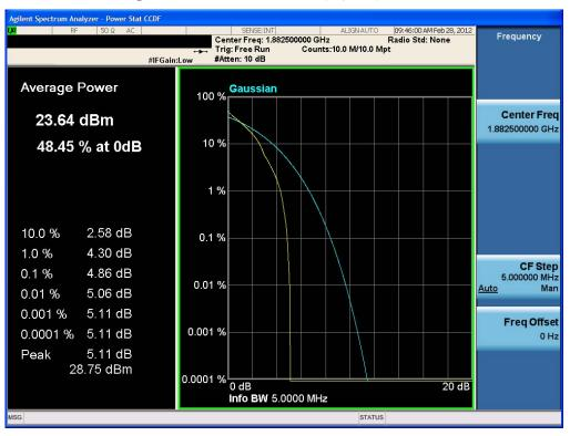
Peak-Average Ratio Plot (5.0 MHz BW, QPSK, Band 25: LOW CH)
