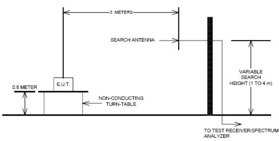
The measurement facilities used for this test have been documented in previous filings with the commission pursuant to section § 2.948. The SAC(Semi-Anechoic Chamber) meets requirements in ANSI C63.4 –2003. A mast capable of lifting the receiving antenna from a height of one to four meters is used together with a rotatable styrofoam platform mounted at three from the antenna mast.
