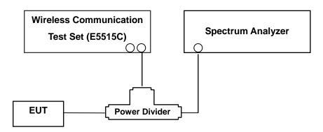
(Configuration of conducted Emission measurement)
