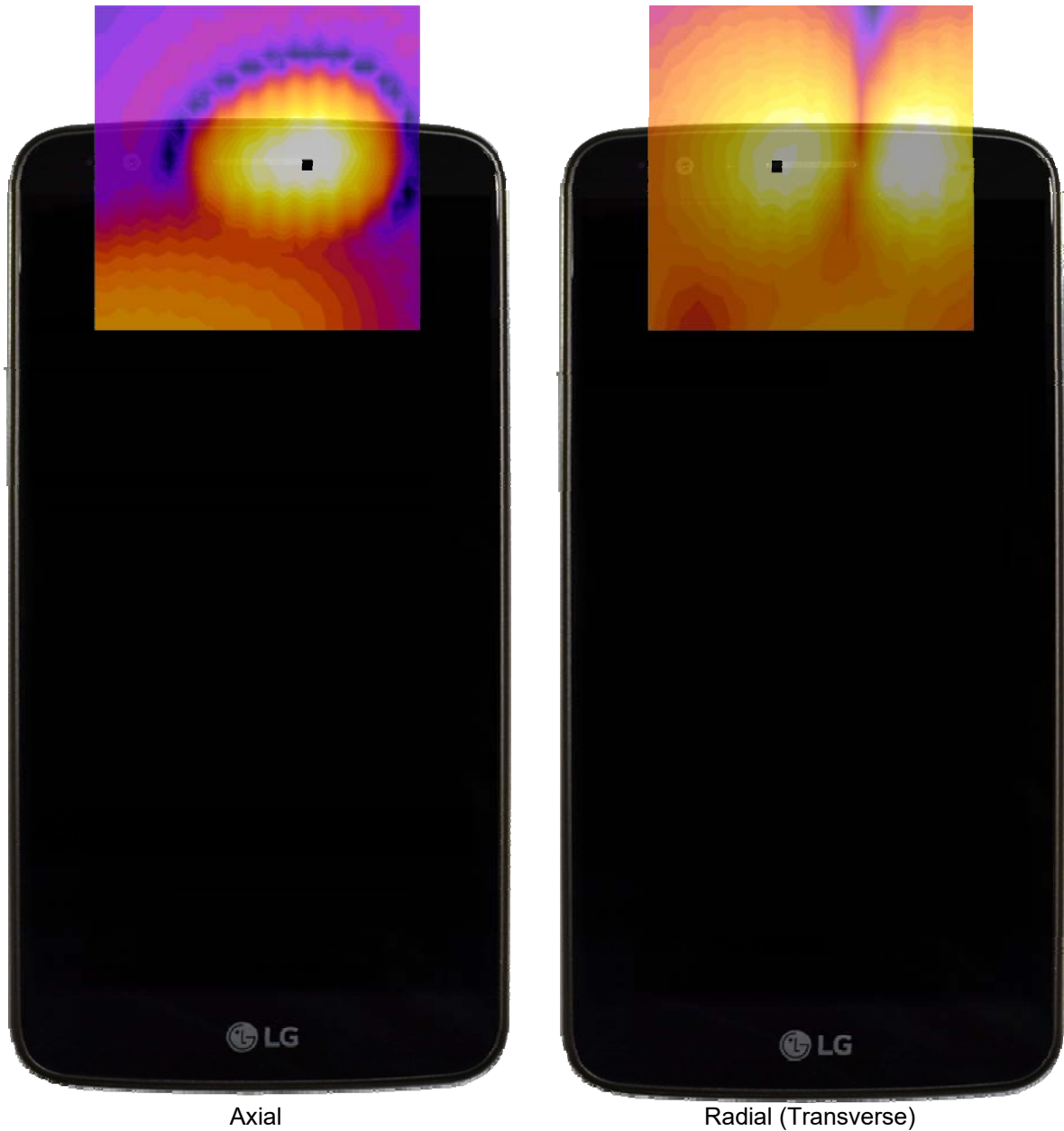
Figure 13-3 T-Coil Scan Overlay Magnetic Field Distributions
