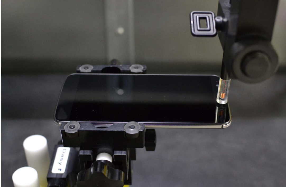
Figure 13-1 Test Setup for Wireless Device
