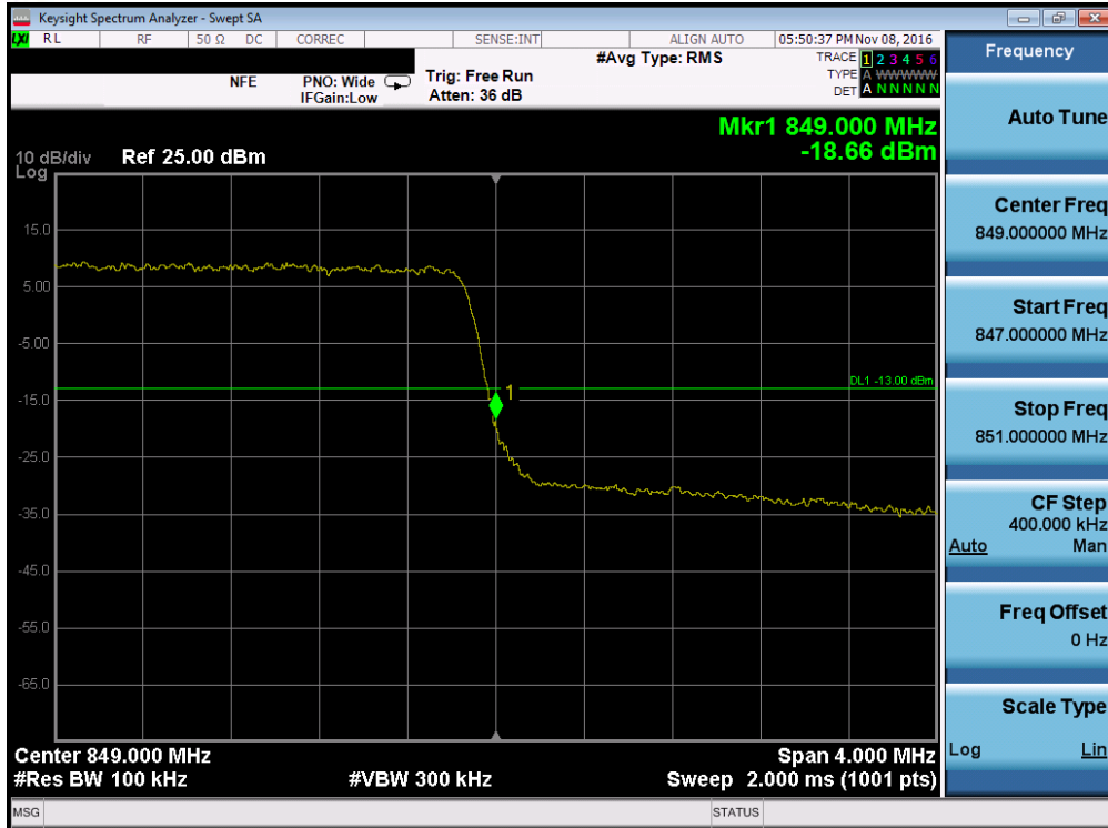
Plot 7-107. Upper Band Edge Plot (Band 26/5 – 3.0MHz QPSK – RB Size 15)
