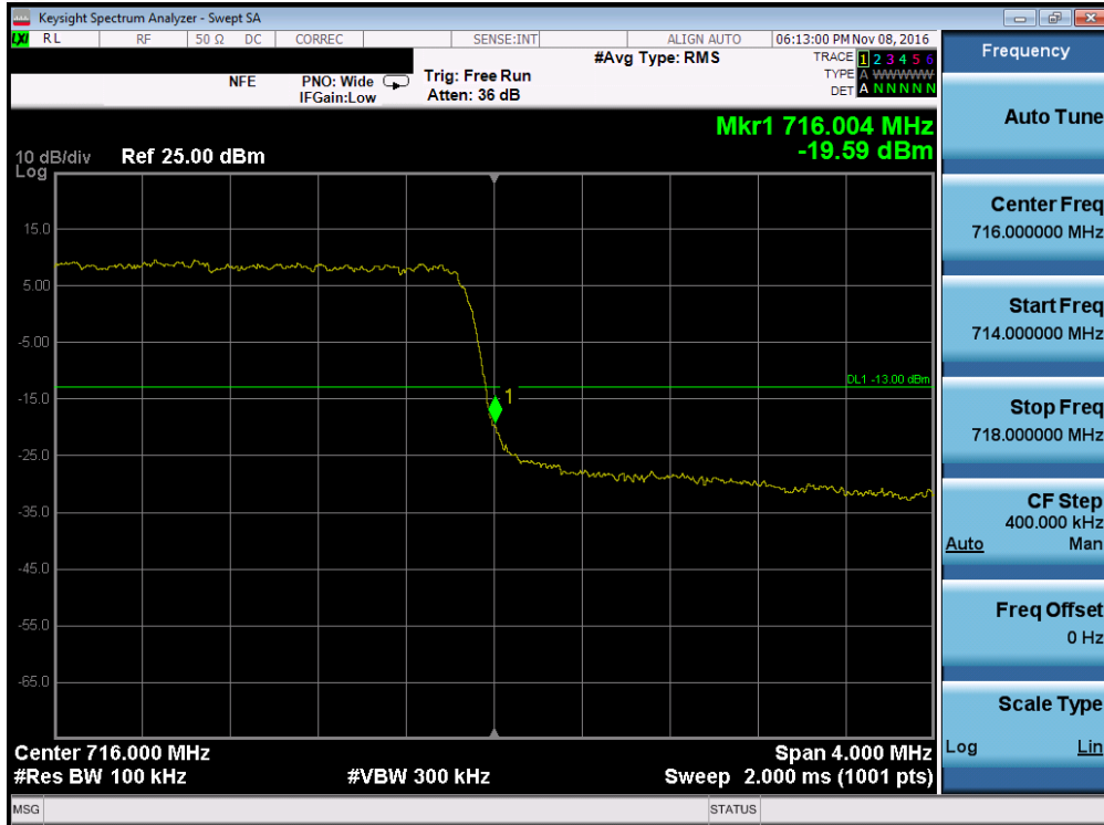
Plot 7-99. Upper Band Edge Plot (Band 12 – 3.0MHz QPSK – RB Size 15)
