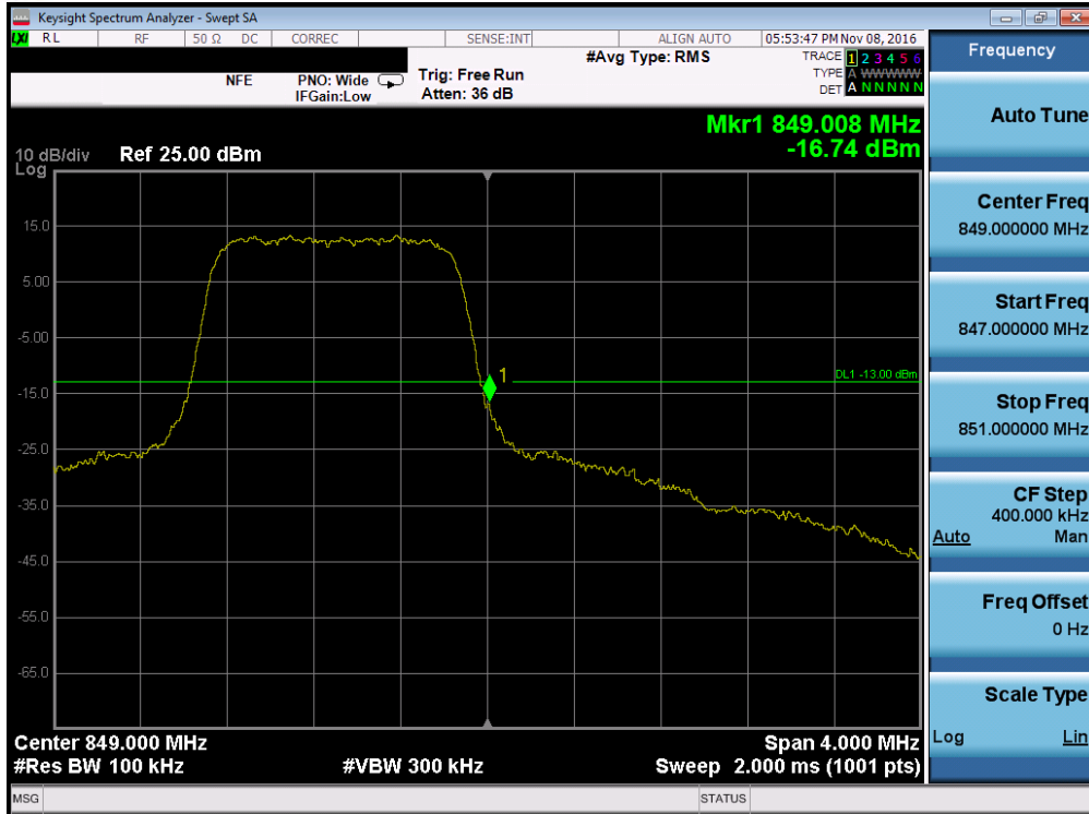
Plot 7-105. Upper Band Edge Plot (Band 26/5 – 1.4MHz QPSK – RB Size 6)
