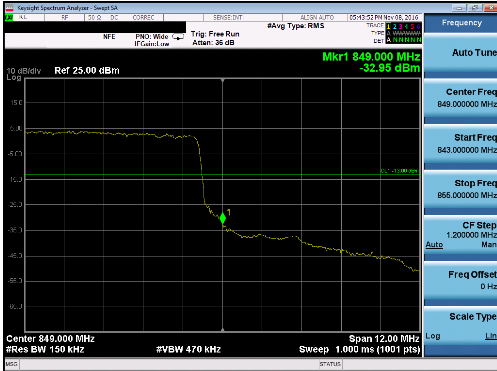
Plot 7-113. Upper Band Edge Plot (Band 26 – 15.0MHz QPSK – RB Size 75)
