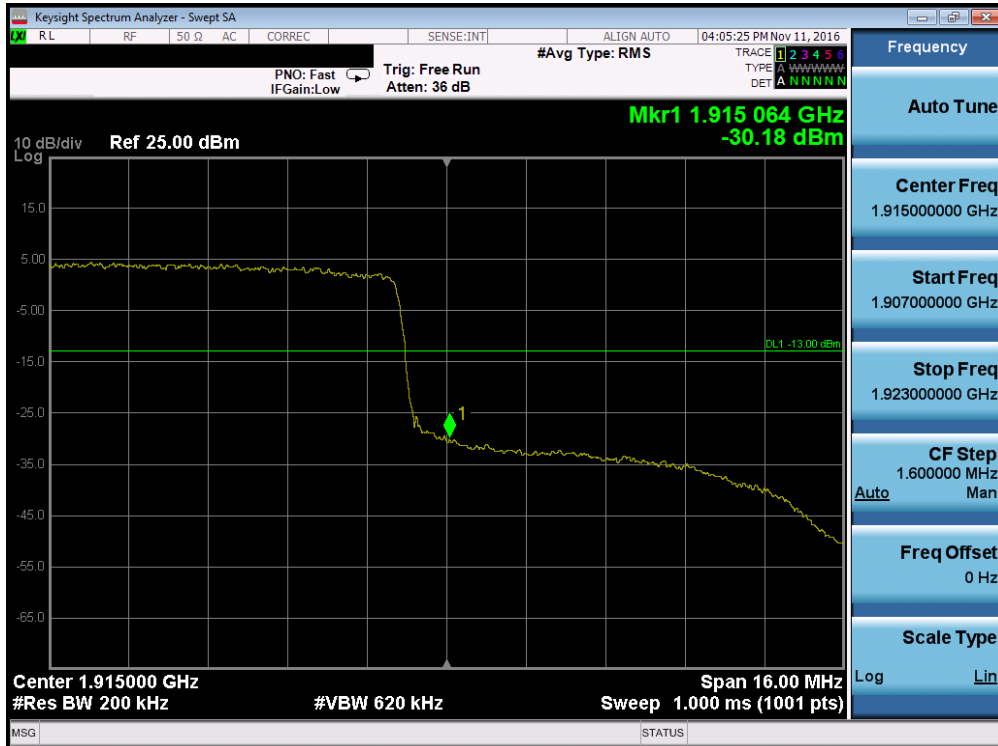
Plot 7-160. Upper Band Edge Plot (Band 25/2 – 20.0MHz QPSK – RB Size 100)
