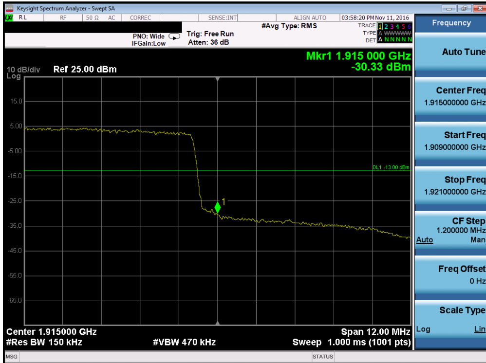
Plot 7-156. Upper Band Edge Plot (Band 25/2 – 15.0MHz QPSK – RB Size 75)
