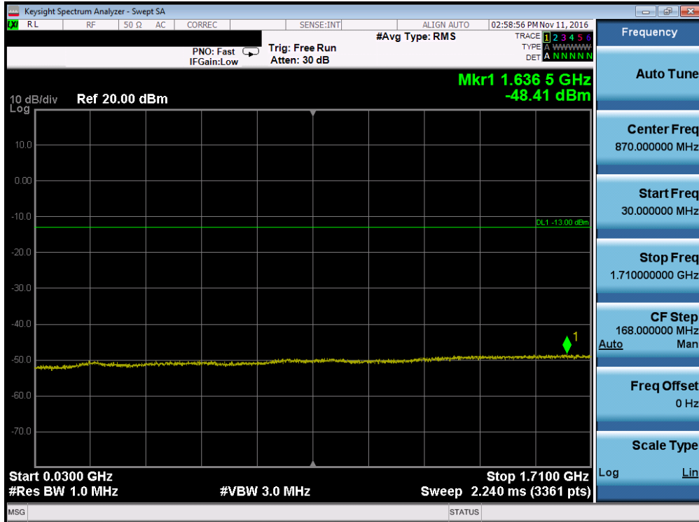
Plot 7-75. Conducted Spurious Plot (Band 4 – 1.4MHz QPSK – RB Size 1, RB Offset 0 – High Channel)
