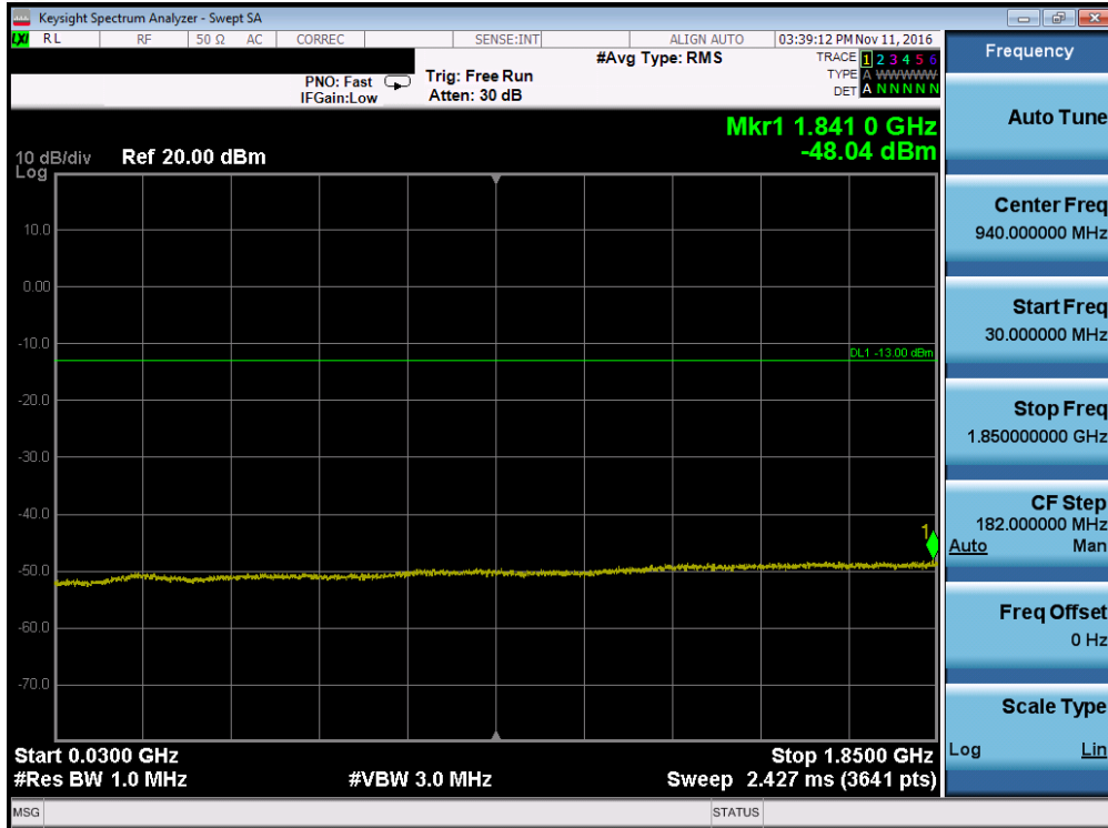
Plot 7-81. Conducted Spurious Plot (Band 25/2 – 3.0MHz QPSK – RB Size 1, RB Offset 0 – Mid Channel)
