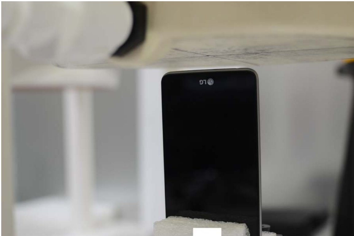
SAR Test Setup Photo 8 – Bottom Edge (10 mm)
