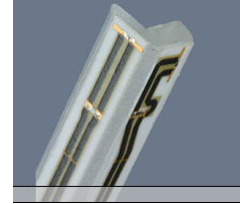
Figure 5-1 E-field Free-space Probe
