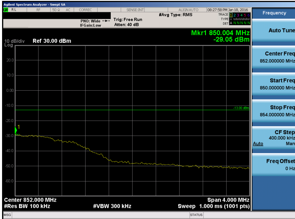
Plot 7-117. Upper Extended Band Edge Plot (Band 5/26 – Band 5 – 3.0MHz QPSK – RB Size 15)
