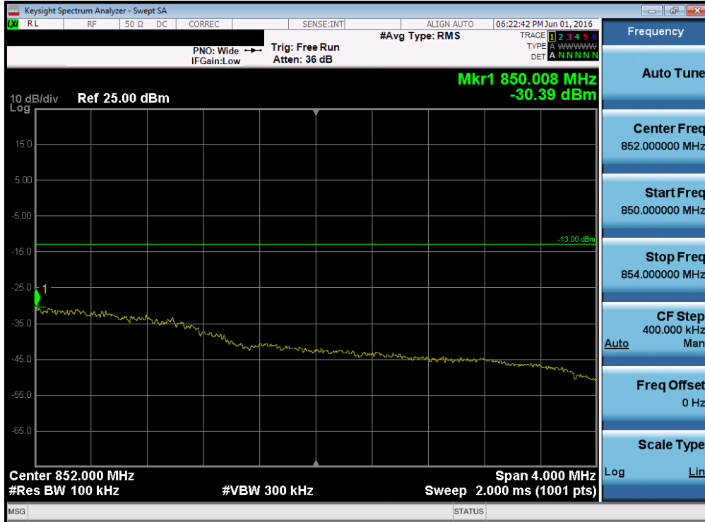
Plot 7-119. Upper Extended Band Edge Plot (Band 5/26 – Band 5 – 3.0MHz QPSK – RB Size 15)
