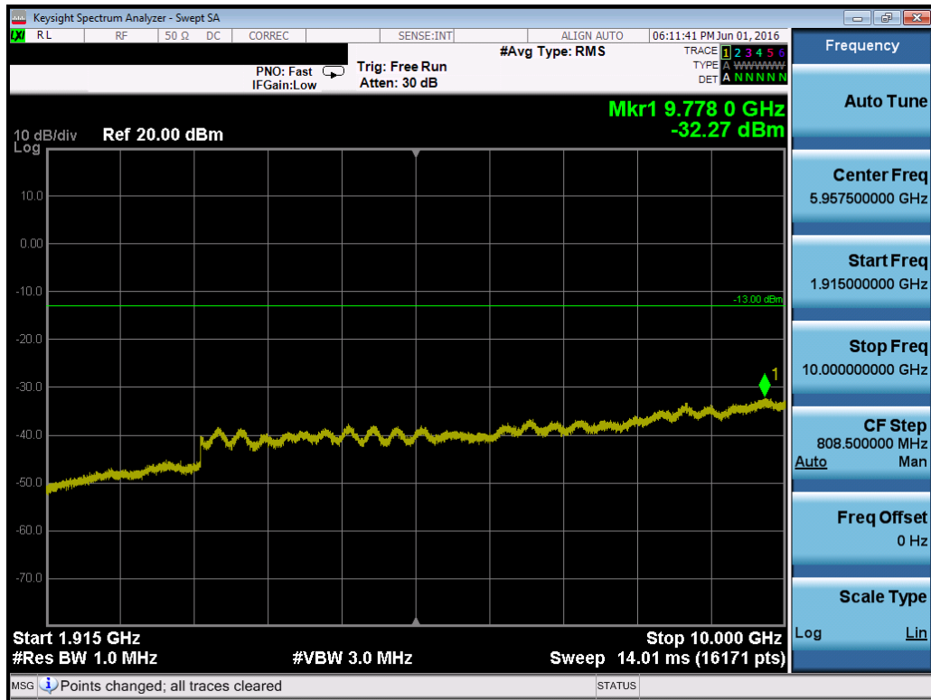
Plot 7-82. Conducted Spurious Plot (Band 25 – 20.0MHz QPSK – RB Size 1, RB Offset 0 – Mid Channel)
