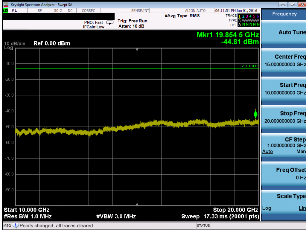
Plot 7-83. Conducted Spurious Plot (Band 25 – 20.0MHz QPSK – RB Size 1, RB Offset 0 – Mid Channel)
