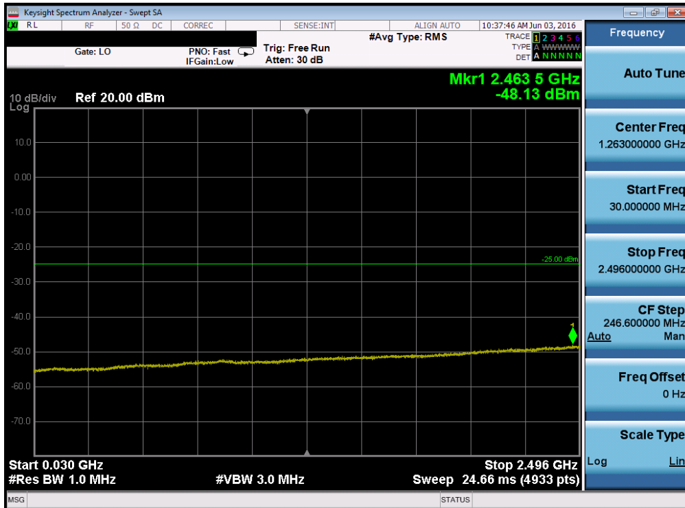
Plot 7-90. Conducted Spurious Plot (Band 41 – 20.0MHz QPSK – RB Size 1, RB Offset 0 – Mid Channel)
