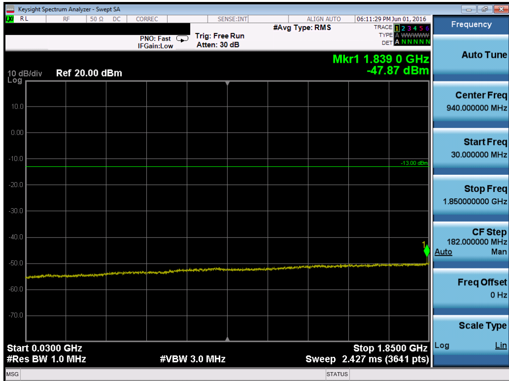
Plot 7-81. Conducted Spurious Plot (Band 25 – 20.0MHz QPSK – RB Size 1, RB Offset 0 – Mid Channel)
