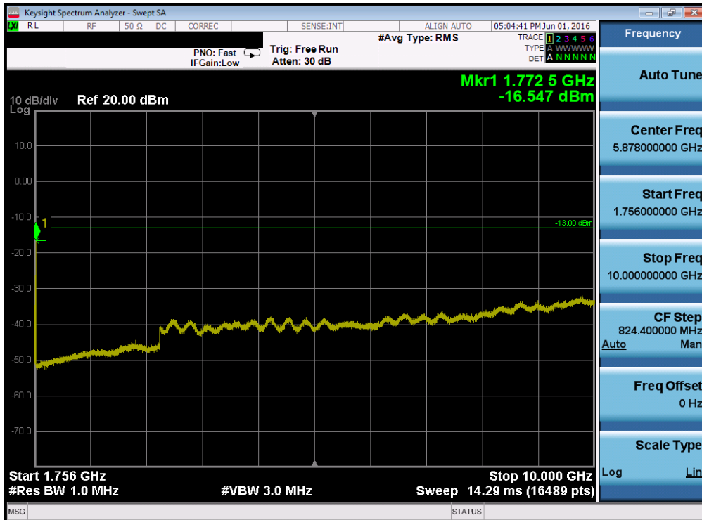
Plot 7-76. Conducted Spurious Plot (Band 4 – 20.0MHz QPSK – RB Size 1, RB Offset 0 – High Channel)
