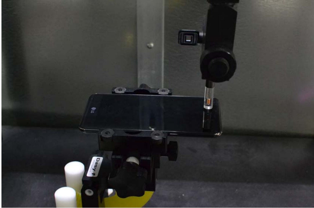
Figure 13-1 Test Setup for Wireless Device
