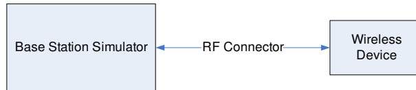
Figure 9-3 Power Measurement Setup
