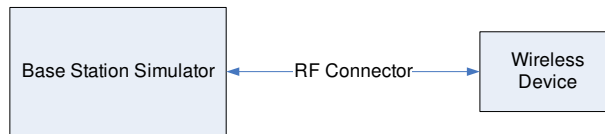
Figure 9-2 Power Measurement Setup
