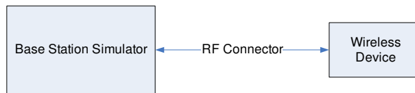
Figure 9-4 Power Measurement Setup
