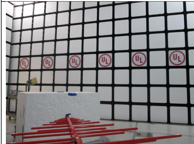
RADIATED FRONT PHOTO (BELOW 1 GHz)
