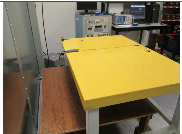
LINE CONDUCTED SIDE VIEW PHOTO
