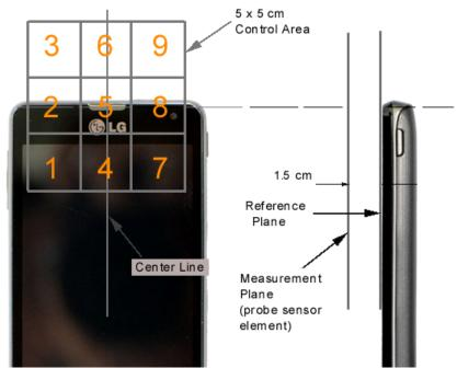
Figure 18-3 5x5 Scan grid above WD
