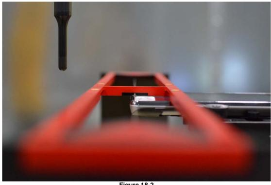
Figure 18-2 HAC Phantom Plane Alignment
